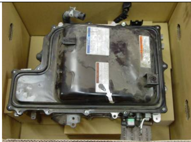
2006 Highlander HV Inverter assembly that set DTC P0A78, illuminated MIL and rendered Vehicle inoperative.
