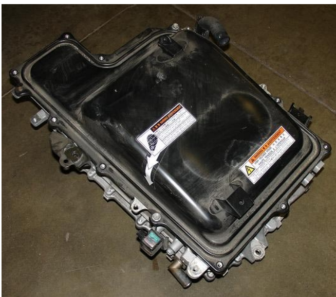
Photo of Inverter Assembly
