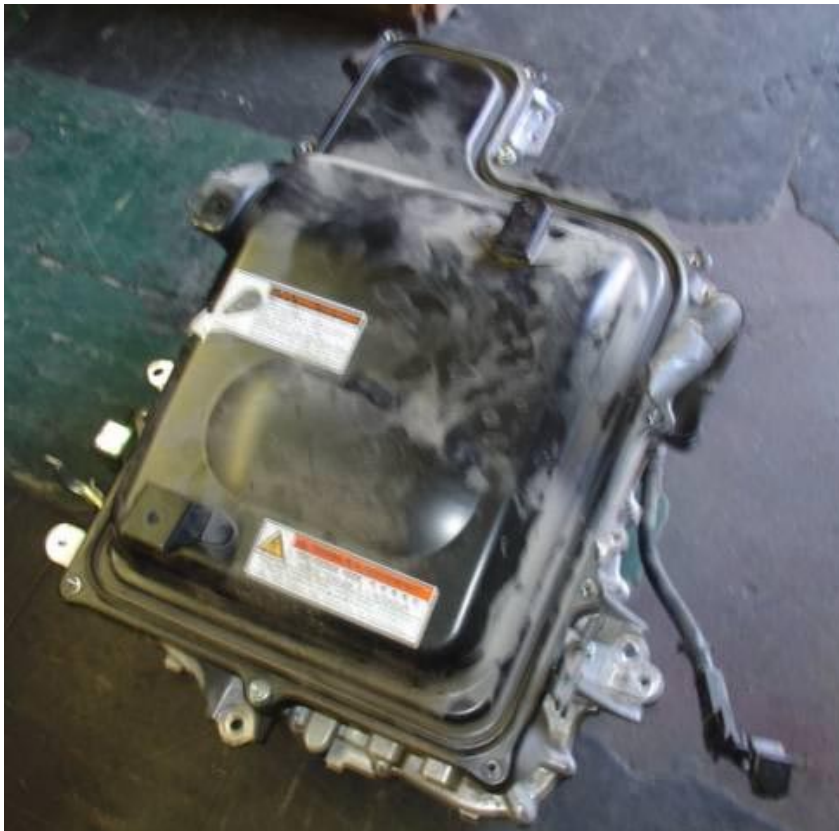
Above: Inverter assembly removed from vehicle.
