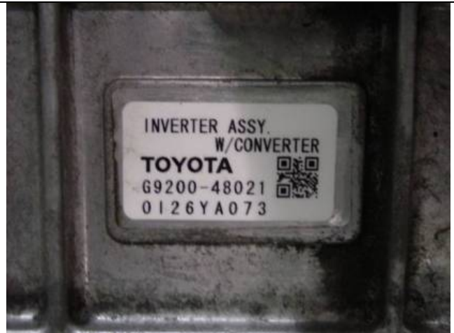
Close-up photo showing manufactures markings on malfunctioning Inverter assembly. Markings were: G9200 – 48021 0126YA073
