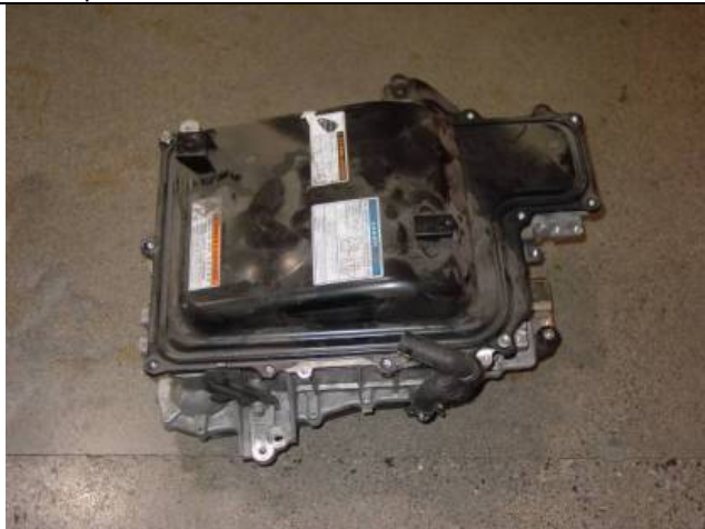
2006 Highlander HV Inverter assembly that set DTC P0A7A, illuminated MIL and rendered Vehicle inoperative.
