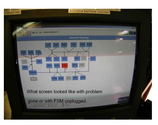
bottom of third seat and the symptoms all went away. After one minute the FSM was plugged back in and immediately all the symtoms came back and all the modules turned red on network topology.
