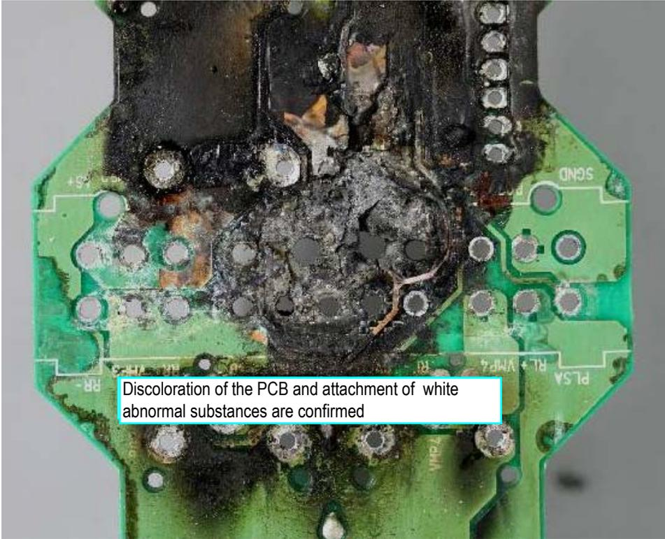
Soldering side of the PCB (With connector base removed)
