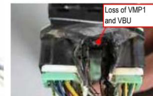
Enlarged connector view of the soldering side
