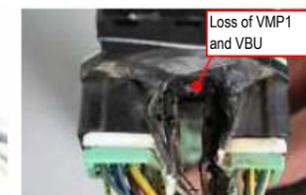
Enlarged connector view of the soldering side
