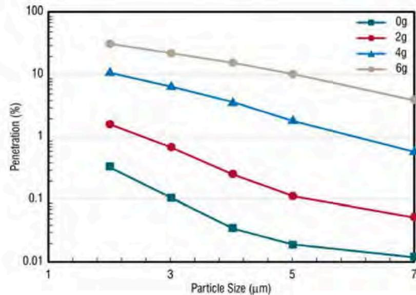
Particle separation for various vibration accelerations, 0g to 6g. Measured with Viscor fluid at 15 Hz
