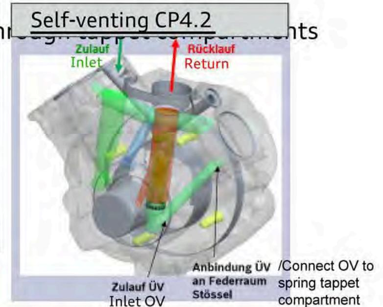
A self-venting CP4.2 improved venting capability to CP4.1 level and further reduced temperature in the drivetrain compartment by ~10K compared to RP2
