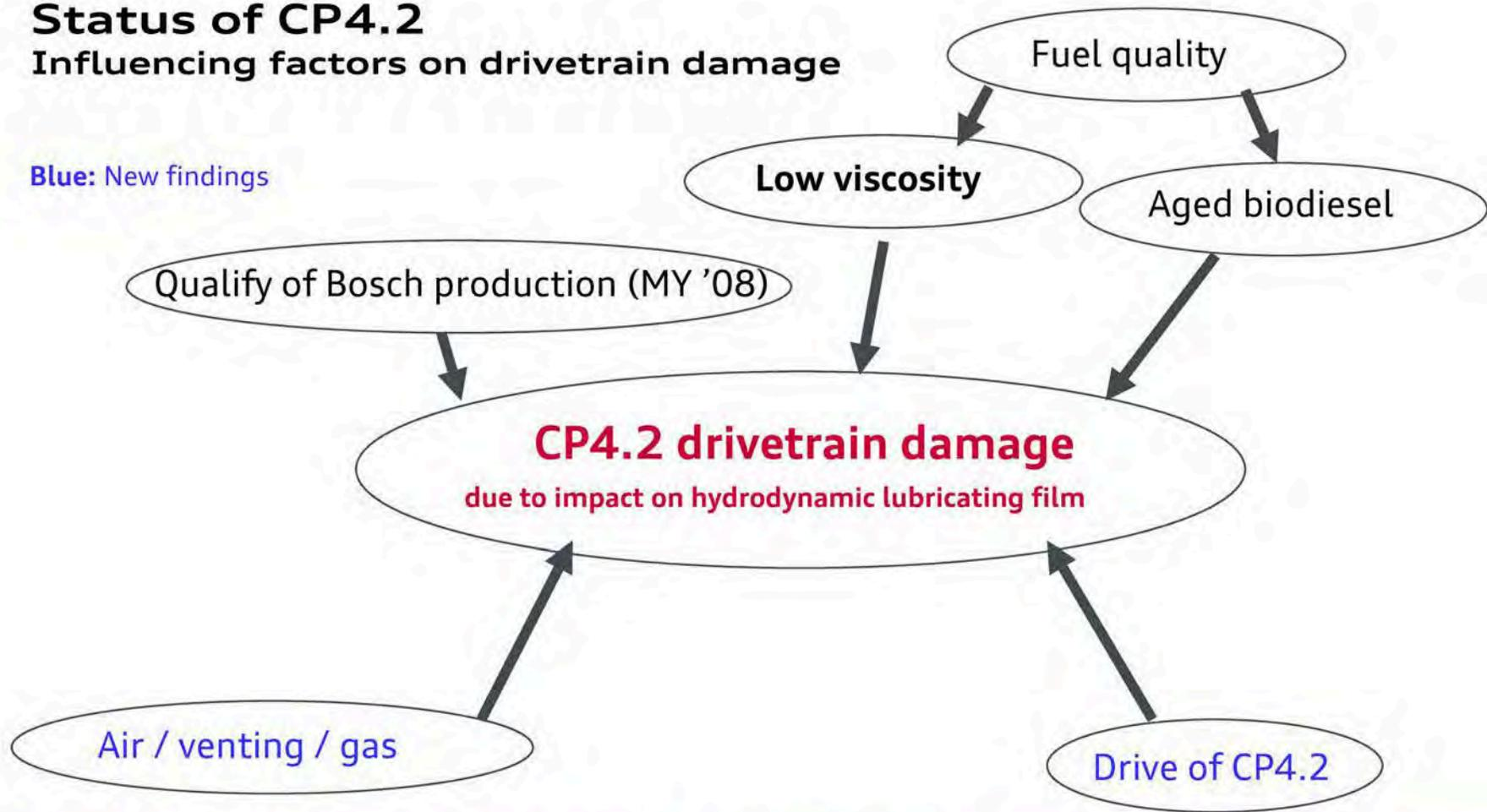
Mixed friction between roller and roller support results in wear of CP4 and must be avoided under all conditions.
