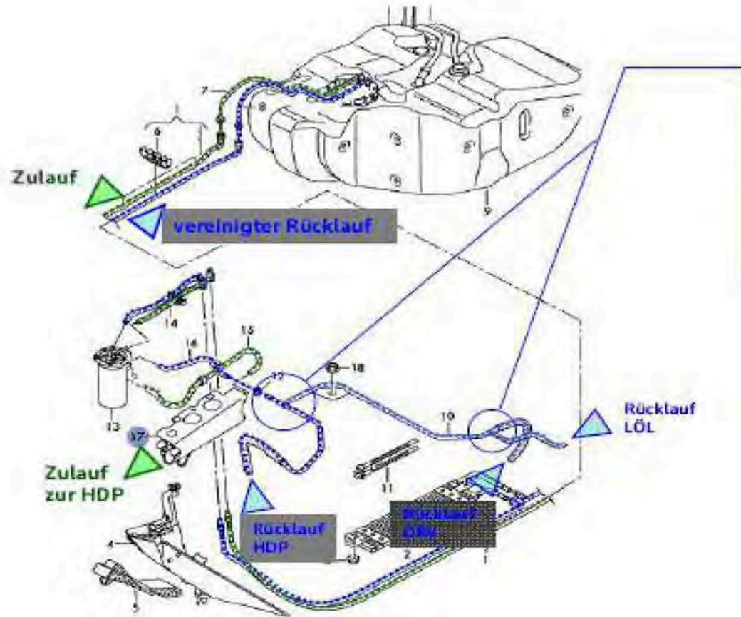
All three return lines together flow back to the tank. Inflow and return lines create a simple flow circuit, which itself ventilates by the operation of the EFP.
