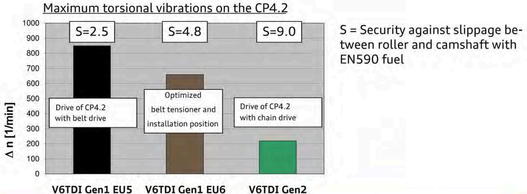
Reducing the torsional vibrations of the CP4.2 reduces the risk of slippage between roller and cam, and thus the danger of flattening
