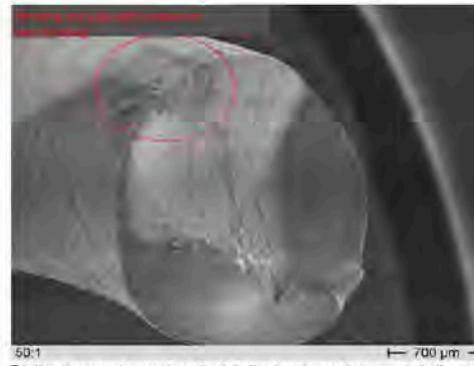
50:1 Friction trace and corrosion attack in the breakage start area (winding top side corrosion attack in the breakage start zone)
