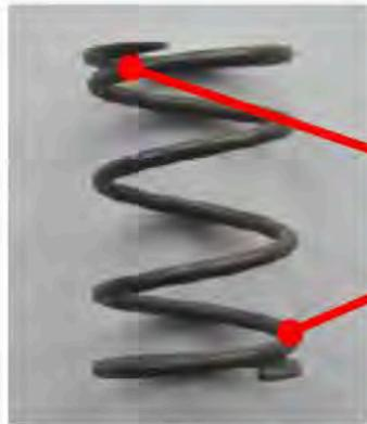
Break location (on both spring ends at times)
