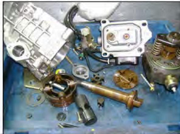
In many cases the fuel pump was failed due to poor quality of DIESEL fuel and presence of moisture / water content.
