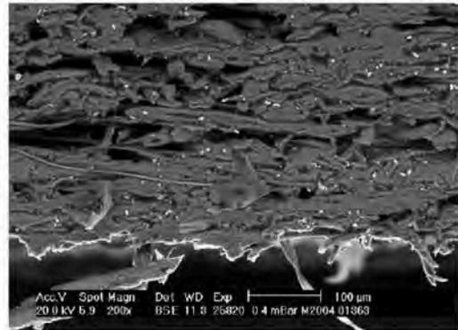
Example for deep filtration with melt-blown paper combination
