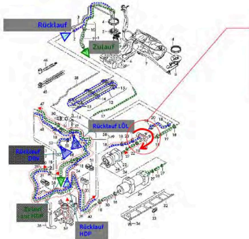
Preheating valve in the LP circuit returns a part of the return flow to the inflow (Quantity depends on the temperature of the diesel). It cannot completely ventilate the LP circuit.
