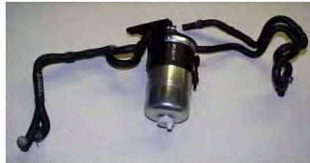
KFD assembly with bracket and fuel tubes
