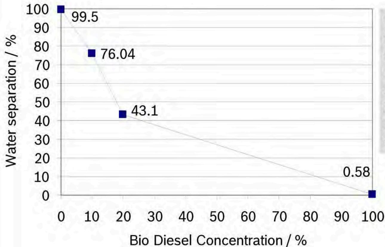
Water separability reduces significantly with increasing Bio Diesel concentration due to reduction of interfacial tension between water and fuel.
