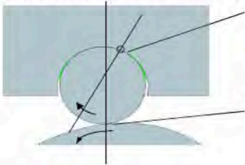
Deposits and / or vapor mixture prevent the buildup of a hydrodynamic pressure, thus no hydrodynamics and a stationary roller
