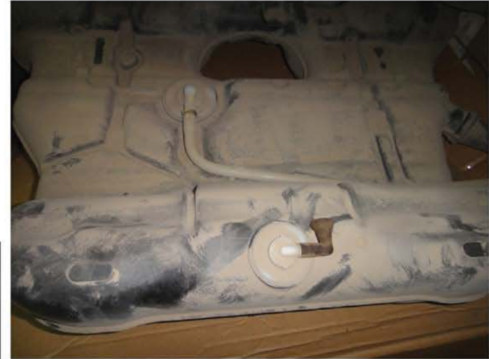
Dust load on dismantled tank
