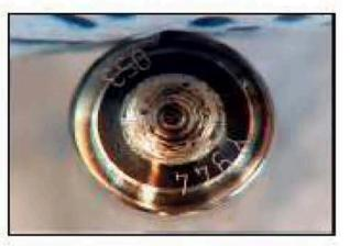
C layer entrained to large extent + abrasive Material wear (or seizing) more than Ø 3mm
