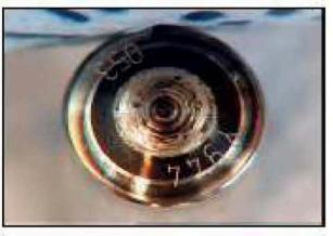
C layer almost completely entrained + abrasive Material wear (seizing) on whole face
