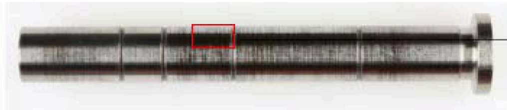
HP pistons with scoring in the circumferential direction on the piston rod
