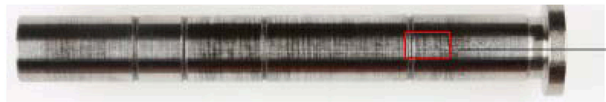
HP piston with corrosion in the up section of the piston rod
