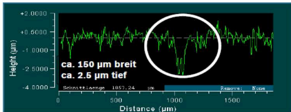
Fig. 5: WLI (white-light interferometry) measurement result, camshaft
