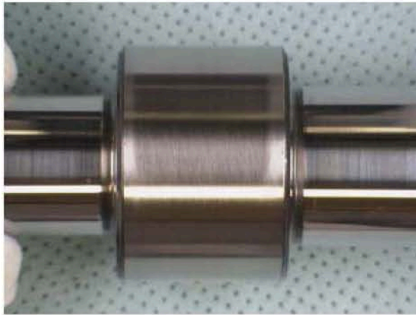
Fig. 7 Camshaft running surface TDC (top dead center)
