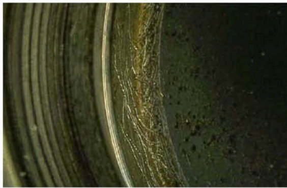
2.008-1206 CR_ARA_M_08_1759 Overview of flange bearing bushing with detached residues
