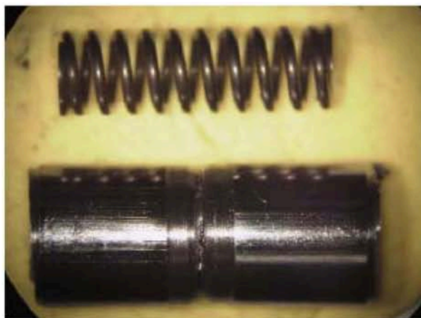
Fig. 11 Non-return valve spring and non-return valve spring seat
