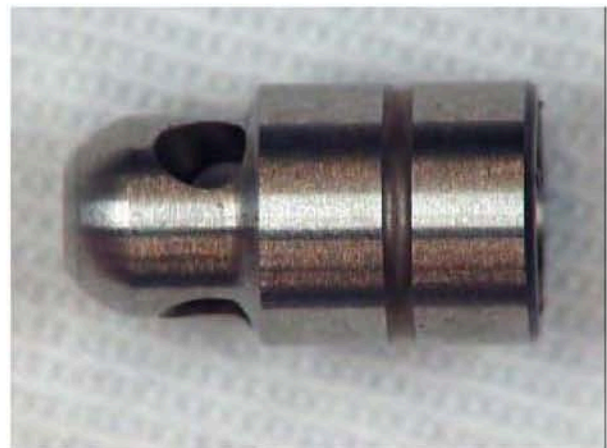
Fig. 10 Non-return valve lateral surface (guidance)
