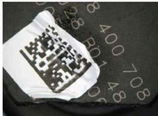
Piece of housing broken without impairment of function
