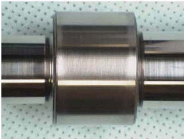
Fig. 7 Camshaft running surface TDC (top dead center)
