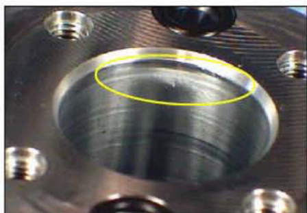
Fig. 3 Housing, tappet hole (cavitation)
