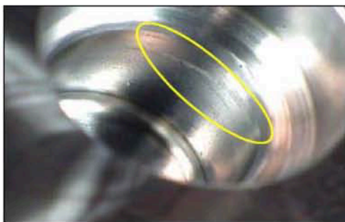
Fig. 1 Housing, metering unit hole (scrape marks)
