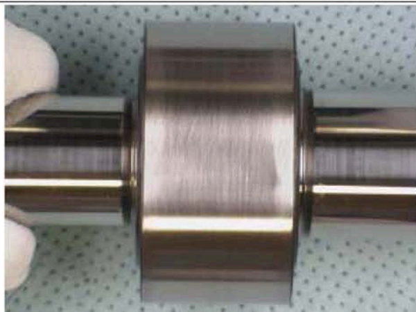
Fig. 6 Camshaft running surface BDC (bottom dead center)
