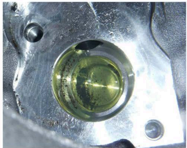
Fig. 2: Dirt, photo of metering unit
