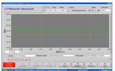
Within a few minutes, considerable rail pressure fluctuations occurred, breakaway torque remaining too high
