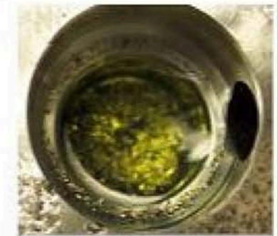
Metal in high pressure pump
