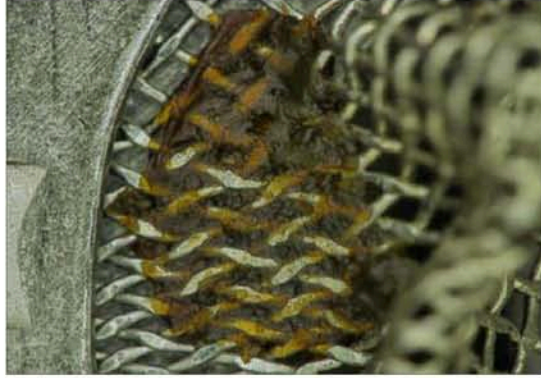
Fig. 14. Overflow valve, screen (covering)
