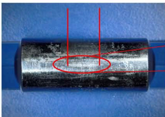
Fig. 3: Roller support, running face with braking flat
