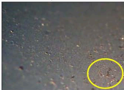
Fig. 14. Detail from Fig. 9, oxidized particles on the surface
