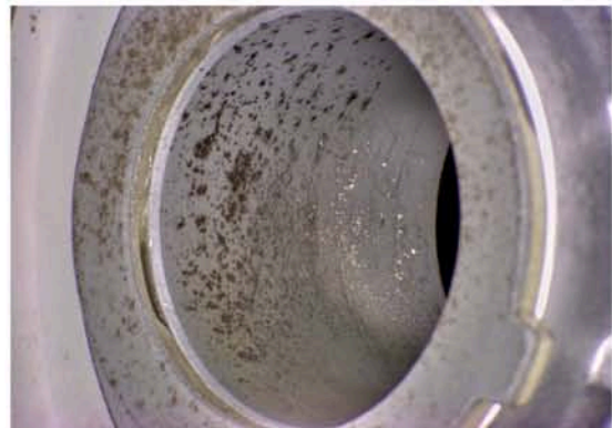
Fig. 8: Flanged bearing bushing, damage caused by particles
