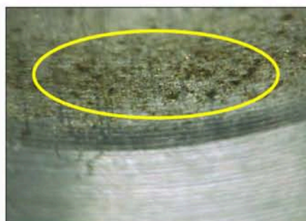
Fig. 18. Tappet borehole, oxidized wear particles
