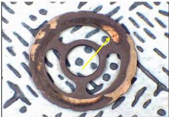
Fig. 7. Spring cup, spring side (oxides)
