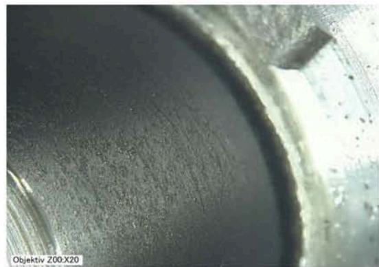
Fig. 10: Housing bearing bushing, damage caused by particles
