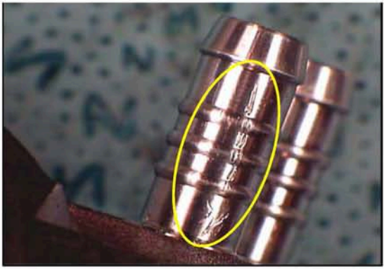
Fig. 7: Return connection (with minor defect)
