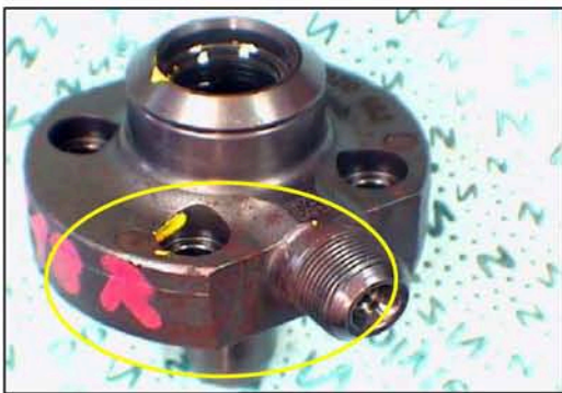
Fig. 2. Cylinder head, surface (rust)
