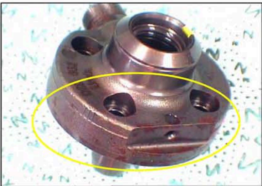
Fig. 3: Cylinder head, surface (rust)
