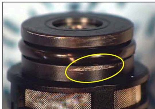
Fig. 12. Metering unit, magnet core on outside (scrape mark)
