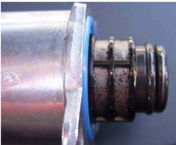
Fig. 1: Dirt in the metering unit
