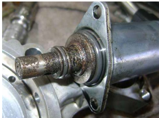
Corrosion fungus and algae growth in secondary fuel filter housing, corrosion bacterial growth on high pressure pump volume control valve.
