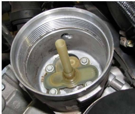
Corrosion in the High Pressure Fuel Pump internal transfer Pump and Secondary Fuel Filter Housing from water in fuel
