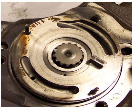
Excessive water in the fuel led to this corrosion in the High Pressure Fuel Pump Internal Transfer Pump and on the Fuel Volume Control Valve
