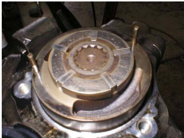
Corrosion in the High Pressure Fuel Pump internal transfer Pump and Secondary Fuel Filter Housing from water in fuel
