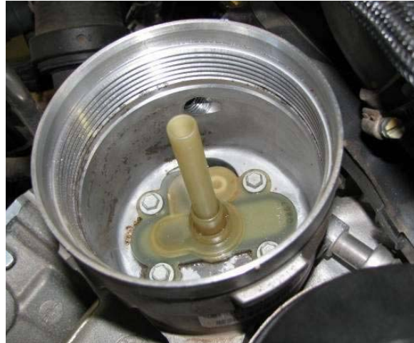
Corrosion in the High Pressure Fuel Pump internal transfer Pump and Secondary Fuel Filter Housing from water in fuel
