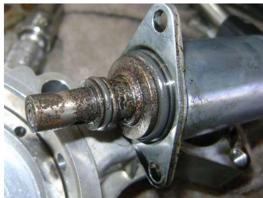
Corrosive fungus, algae and bacterial growth in secondary fuel filter housing and high pressure pump volume control valve.
