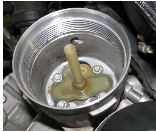
Corrosion in the High Pressure Fuel Pump internal transfer Pump
