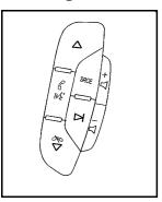
For vehicles with audio steering wheel controls, some audio controls can be adjusted at the steering wheel.
