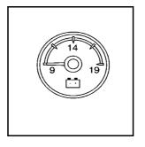
For vehicles with a voltmeter gauge, this gauge indicates the battery voltage when the ignition is turned on.
