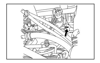
The remote negative (-) terminal is a stud located on the right front passenger side of the engine, where the negative battery cable attaches. See Engine Compartment Overview on page 6-16.
