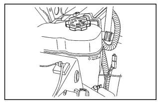
The coolant level should be at or above the FULL COLD mark. If it is not, you may have a leak in the cooling system.
