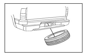
Tilt the tire toward the vehicle with some slack in the cable to access the tire/wheel retainer. Separate the retainer from the guide pin by sliding the retainer up the pin while pressing down on the latch.
