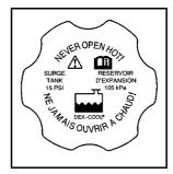
Remove the coolant surge tank pressure cap when the cooling system, including the coolant surge tank pressure cap and upper radiator hose, is no longer hot. Turn the pressure cap slowly counterclockwise about one full turn. If you hear a hiss, wait for that to stop. A hiss means there is still some pressure left.
