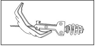
Once the retainer is separated from the guide pin, tilt the retainer and pull it through the center of the wheel along with the cable and guide latch.
