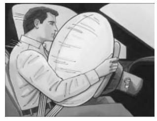
The driver airbag is in the middle of the steering wheel.
