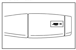
Vehicles with an automatic transmission have a tow/ haul mode. The tow/haul mode adjusts the transmission shift pattern to reduce shift cycling, providing increased performance, vehicle control, and transmission cooling when towing or hauling heavy loads.
