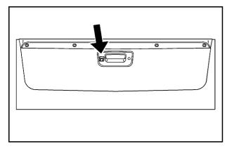
The image is provided by the camera located in the bezel for the tailgate handle.
