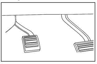
Set the parking brake by holding the regular brake pedal down, then pushing down the parking brake pedal. If the ignition is on, the brake system warning light will come on. See *Brake System Warning Light on page 4-37*.
