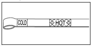
5. Safe operating level is within the HOT cross hatch band on the dipstick. If the fluid level is not within the HOT band, and the transmission temperature is between 71°C and 93°C (160°F and 200°F), add or drain fluid as necessary to bring the level into the HOT band. If the fluid level is low, add only enough fluid to bring the level into the HOT band. It does not take much fluid, generally less than 0.5 Liter (1 Pint). Do not overfill.
