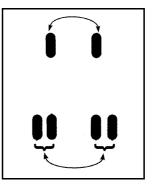
If your vehicle has dual rear wheels and the tread design for the front tires is different from the dual rear tires, always use the correct rotation pattern shown here when rotating the tires.
