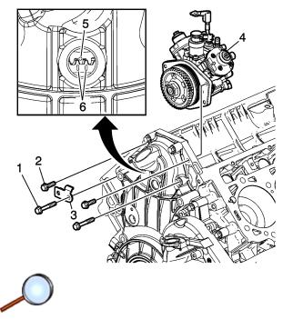
**Note:** The fuel pump must be correctly timed to the camshaft gear.
