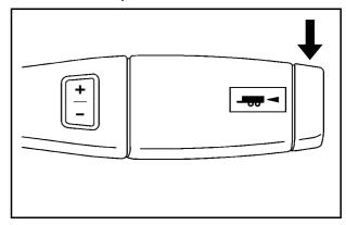
Vehicles with an Allison or Hydra-Matic<sup>®</sup> 6-speed automatic transmission<sup>®</sup> have a tow/haul mode. The tow/haul mode adjusts the transmission shift pattern to reduce shift cycling, providing increased performance, vehicle control, and transmission cooling when towing or hauling heavy loads.
