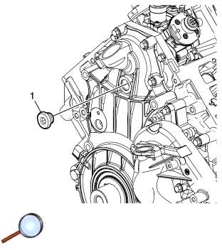
6. Install the camshaft gear access hole plug (1).
