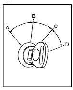
The ignition switch has four different positions.
