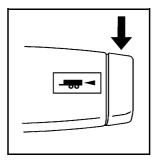
Pressing this button at the end of the shift lever turns on and off the tow/ haul mode.
