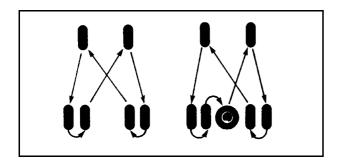
If your vehicle has dual rear wheels and the tread design for the front tires is the same as the rear tires, always use one of the correct rotation patterns shown here when rotating the tires.
