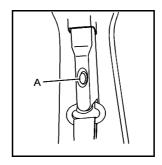
On the extended cab, push down on the release button (A) and move the height adjuster to the desired position.
