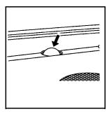
The solar sensor, located in the defrost grille, in the middle of the instrument panel, monitors the solar heat. Do not cover the solar sensor or the system will not work properly.
