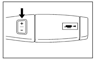
The vehicle may have a Range Selection Mode. The Range Selection Mode helps control the vehicle's transmission and vehicle speed while driving down hill or towing a trailer by letting you select a desired range of gears.
