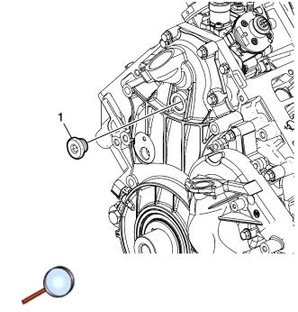
7. Remove the camshaft gear access hole plug(1).
