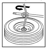
Use the wheel wrench hook which allows you to pull the hoist cable towards you to assist in reaching the spare tire.
