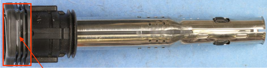
Putty protruded into housing ribs
