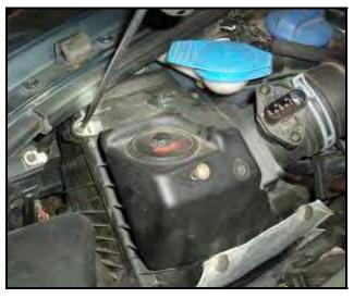
Loosen four screws at each corner of air box cover, and remove air box cover from vehicle
