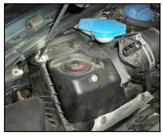
Loosen four screws at each corner of air box cover, and remove air box cover from vehicle
