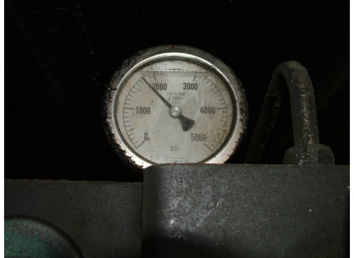
Bus 17 CNG tank Pressure @ 1760 psi
