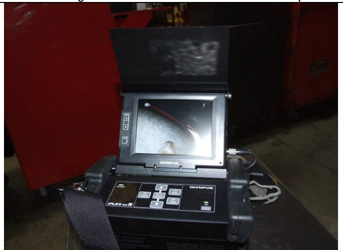
Borescope Used in Inspection of Bus 34 in Garage
