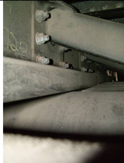
Typical Tank Clearance on Bus 17
