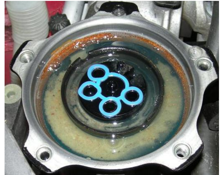
Unknown Deposits, to be analysed (Fuel filter from failed HPFP)
