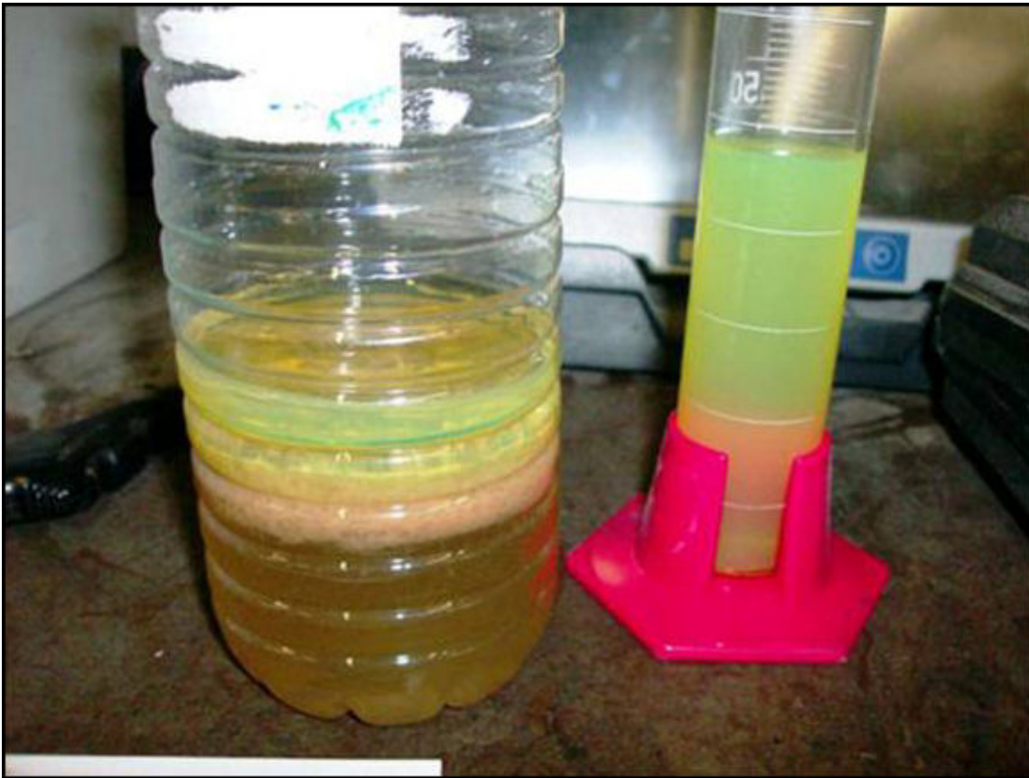
Figure 3. Fuel in the left container is contaminated.
