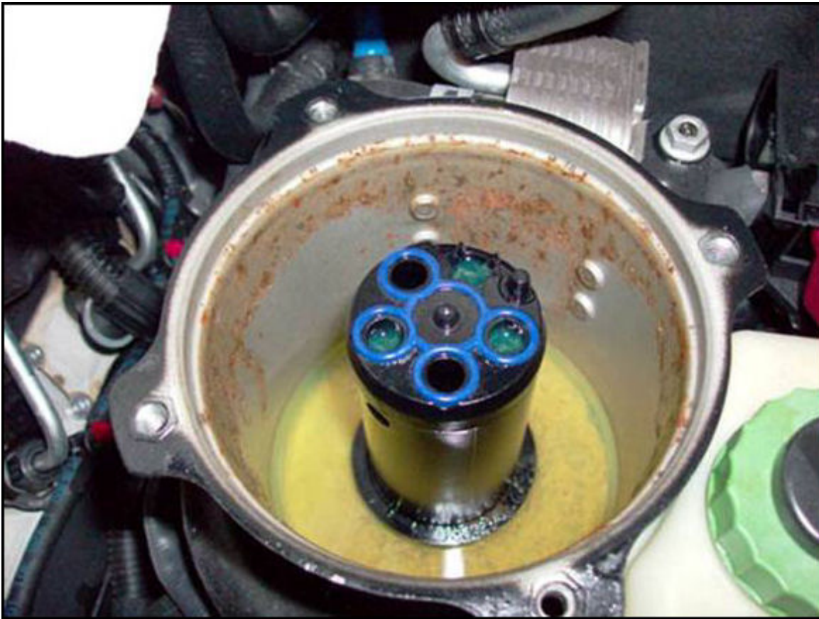
Figure 2. Example of rust in fuel system.
