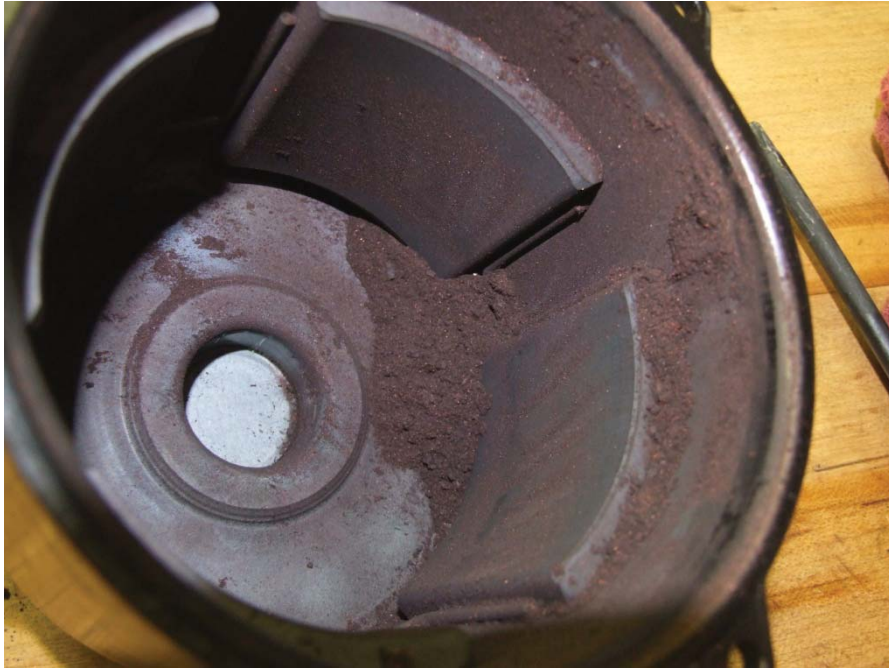
Figure 4 Dust in Motor after Disassembly
