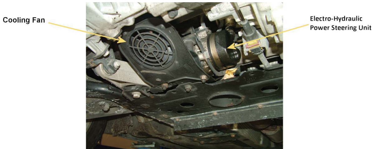
Figure 1 Power Steering Unit and Cooling Fan Mounted in Vehicle
