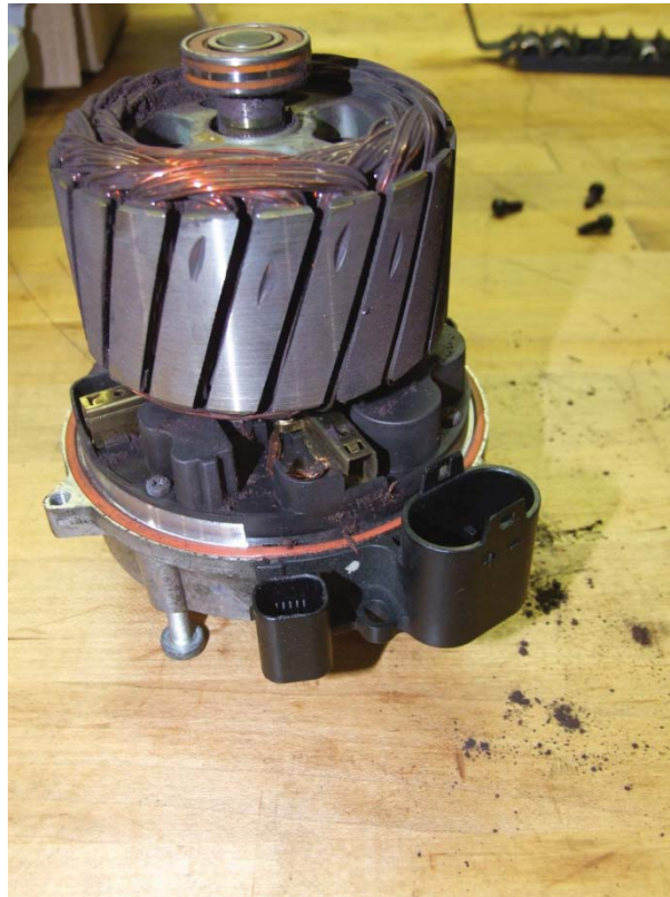
Figure 5 Armature and Electrical Connections
