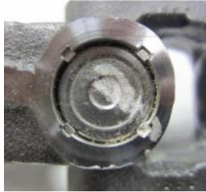
2. Visually check that the steering column and the U joint are properly connected as shown in the picture on the right.
