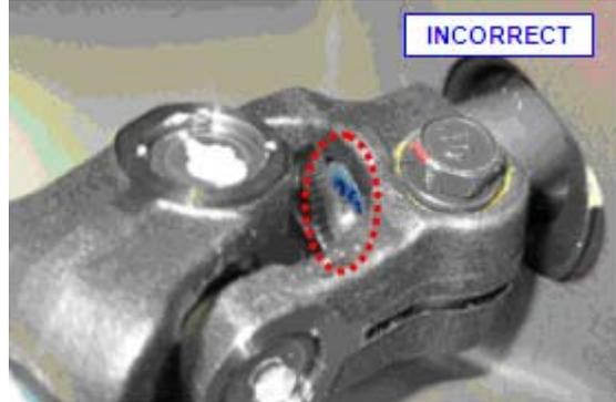
5. Remove the steering column-to-U joint bolt.
