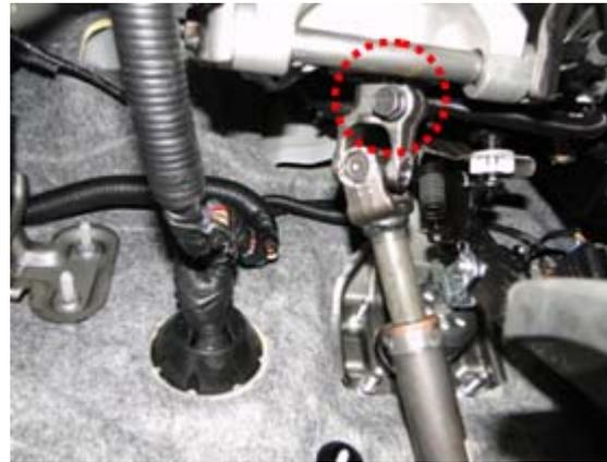
8. Torque the steering column-to-U joint bolt to **39.8~47.0 lb-ft, (53.9~63.7 N-m, 5.5~6.5 kgf-m)** with a torque wrench.
