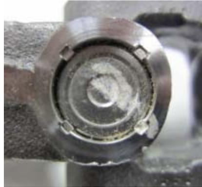
2. Visually check that the steering column and the U joint are properly connected as shown in the picture on the right.
