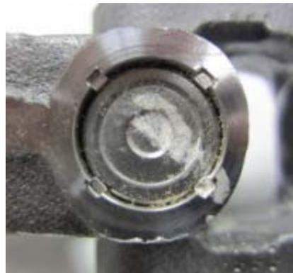
3. Visually check that the steering pinion splined shaft and the U joint are properly connected as shown in the picture on the right.
