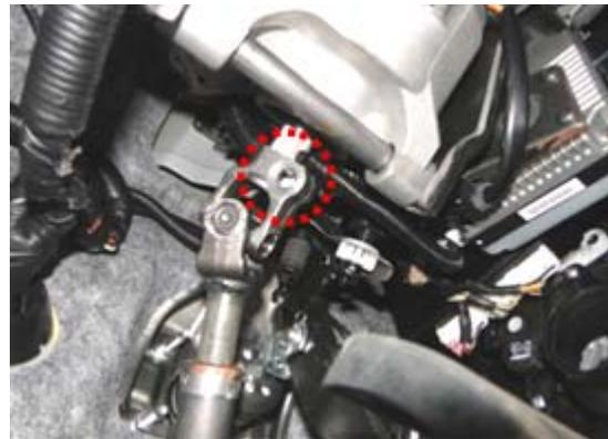
5. Inspect the bolt for damage/ stripping/cross-threading. Inspect the corresponding threads in the U-joint. Replace both if damage is found.
