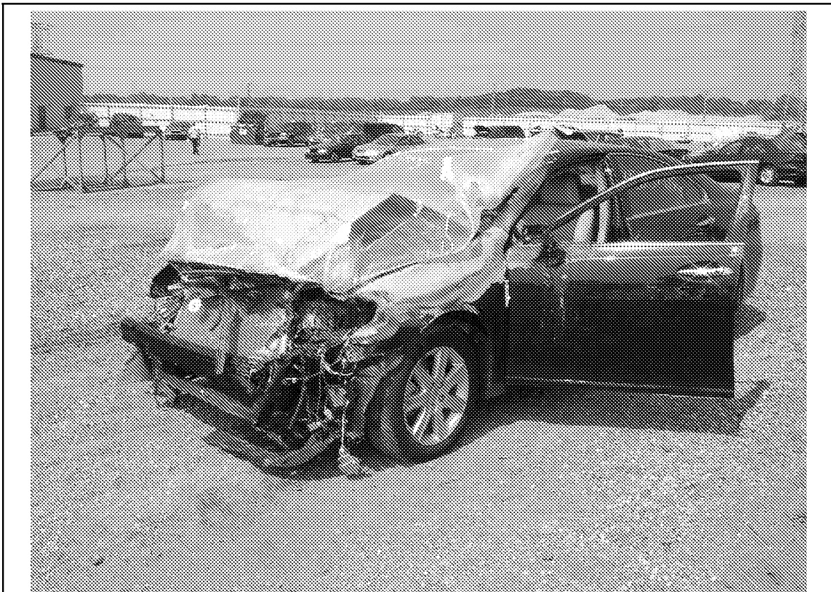
Photo 2: Front oblique view of vehicle showing collision and fire damage
