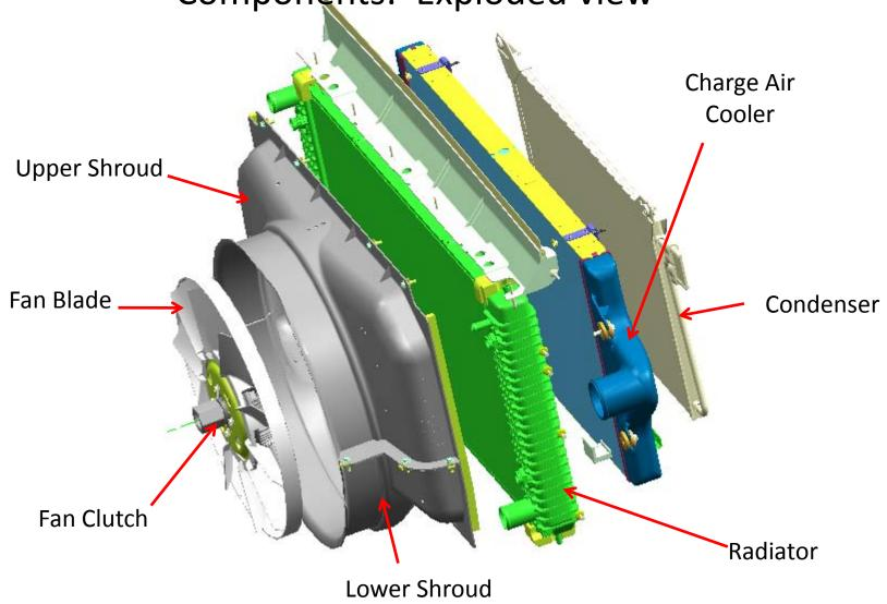
2006 MY L18 Engine Cooling Fan and Related Components: Isometric view
