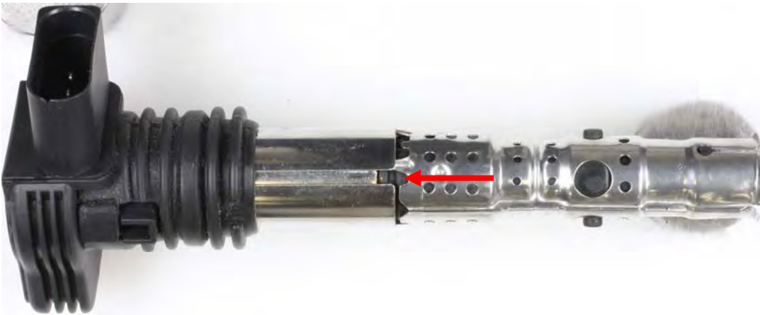
Image 4: coil -3 gap on the return plate moved by 130°
