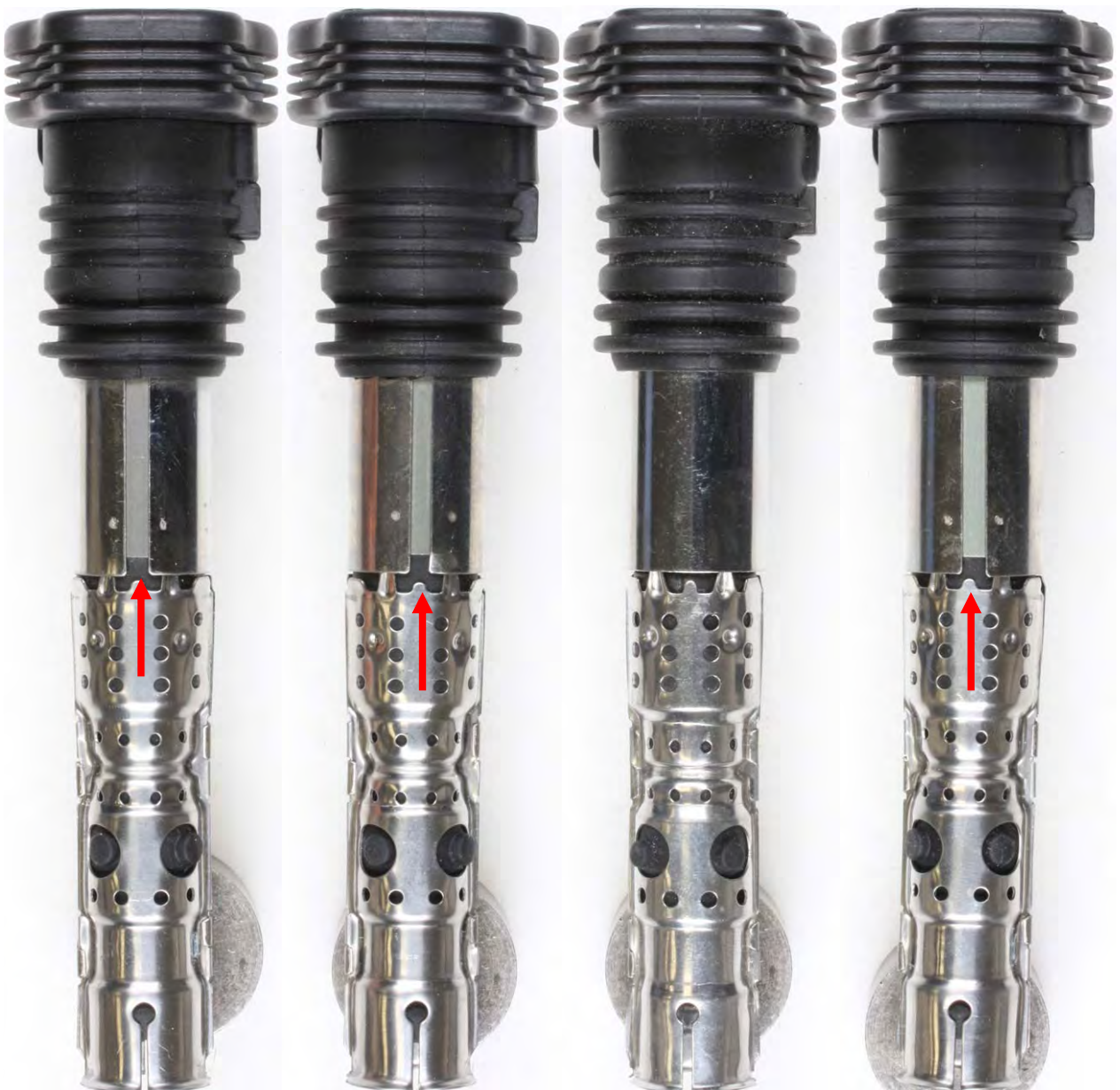
Image 3: coil overview, mark: varying position of the return plate
