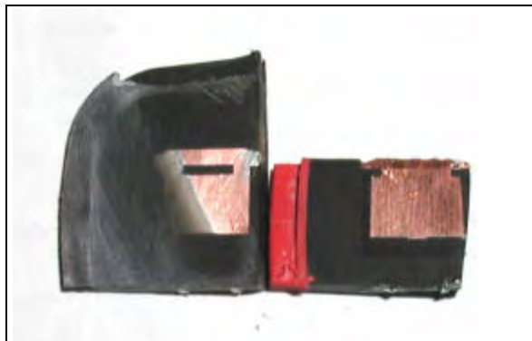
Image of leadframe from both devices after mechanical grind. Device on left is ChipPAC's leadframe while the device on the right is from Cebu.
