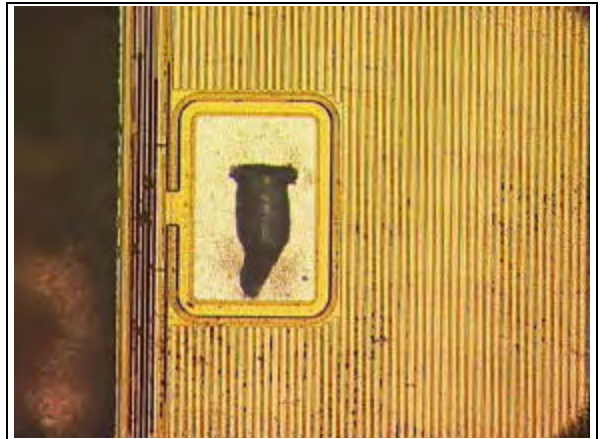
Ref VW – 26-2005-04-12-p-001 Figure 2: Ring area near gate pad showing continued carbonized epoxy left in the ring area after decap. Note black lines in rings and around gate pad, this is carbonized epoxy.
