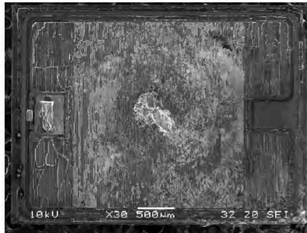
Figure 6: SEM overview of the massive electrical/thermal damage on the die & wires.
