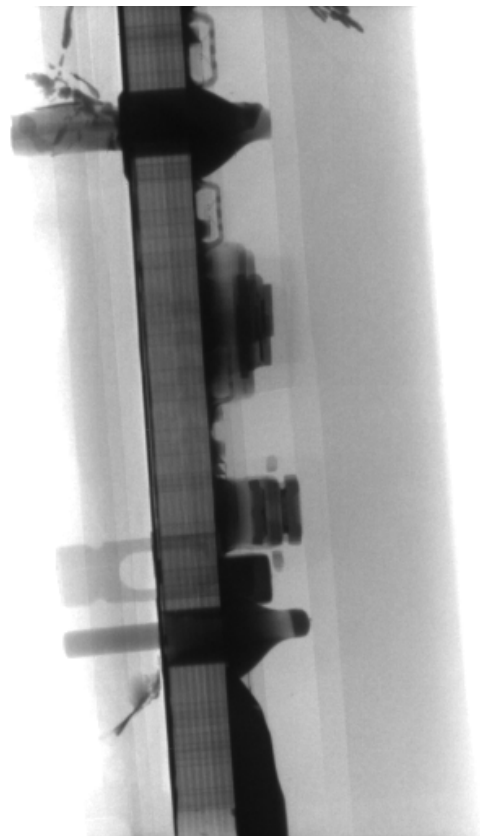
Image 9: Radioscopy image, ignition coil, vehicle ID.3VWSF71K55M603138 Jetta USA,
