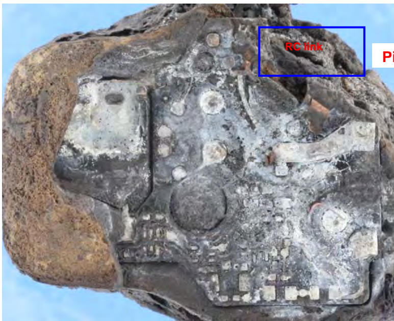
Image 11: 11-z-10-02246_10, damage to the coil head in the area of the RC link
