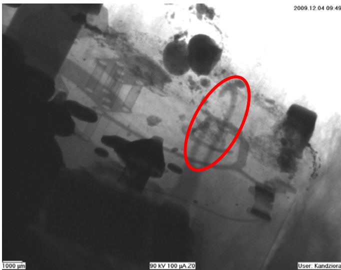
Image 6: printed circuit, RC link area with earth spring: partial destruction of the earth spring in the printed circuit hole.
