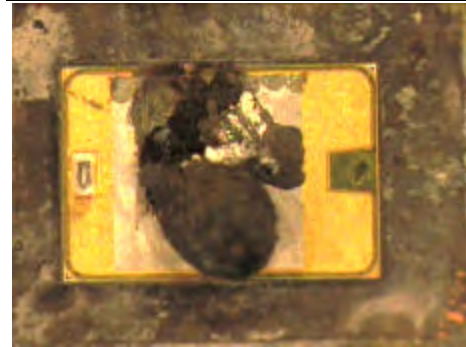
Figure 2: #6476 Electrical damage centered near the emitter bond wire area.
