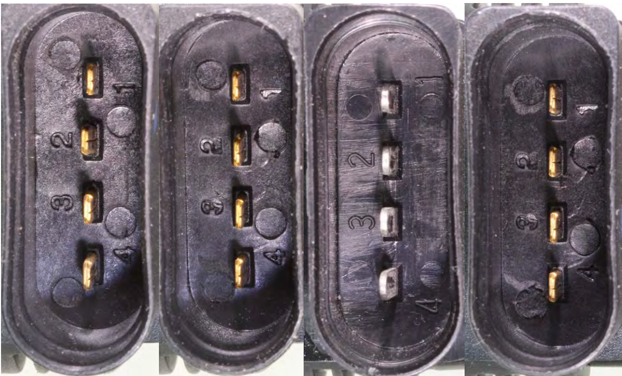
-1 -2 -3 -4 Contacts on brass brass tin-plated brass Image 5: plug
