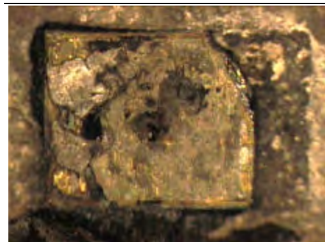
Figure 4: #6423 Electrical damage noted covering the entire die surface.
