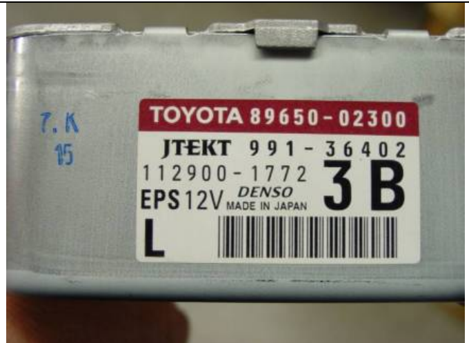
Photo of manufactures markings on EPS ECU. Markings were:
