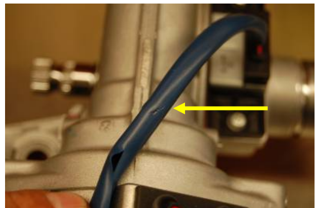
Location of pinch mark on Blue Harness Cover.
