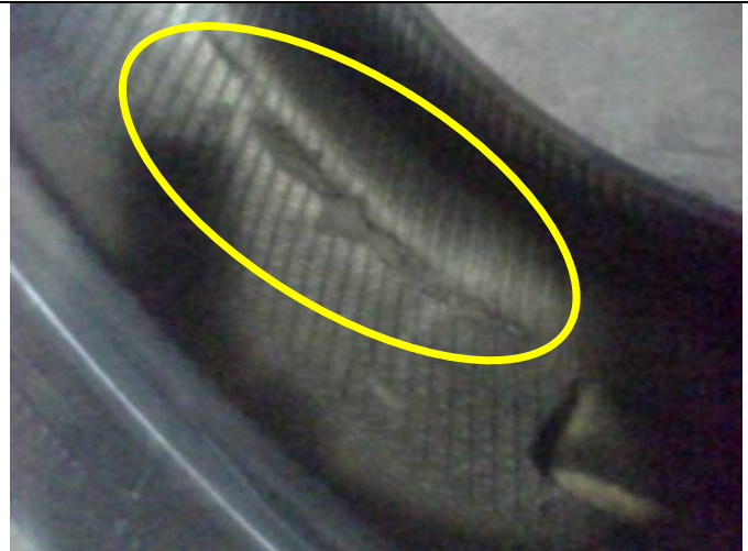
Picture Of Damage Caused By Piece Of Wood
