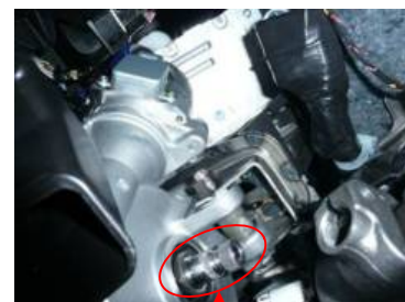
"Play" in internal steering's column shaft
