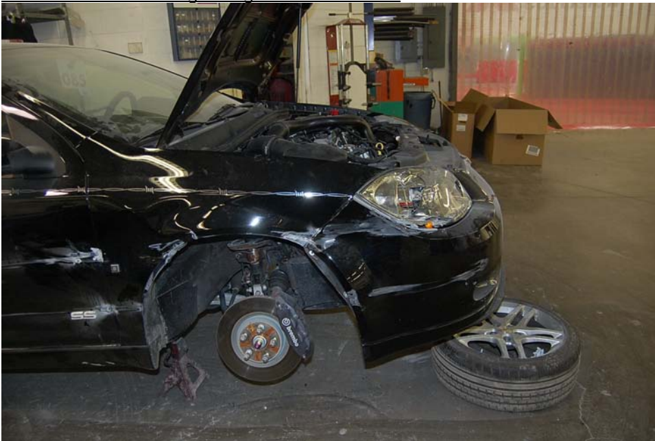
29. Side damage to right fender forward of wheel position.
