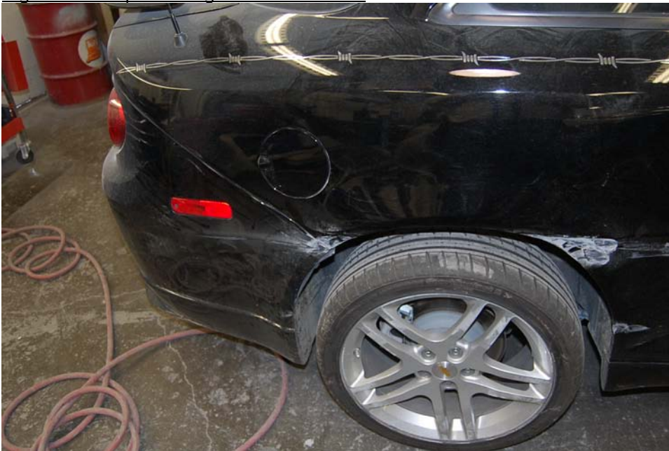
35. Rear bumper overview reveals no damage at face only side damage at extreme right corner.
