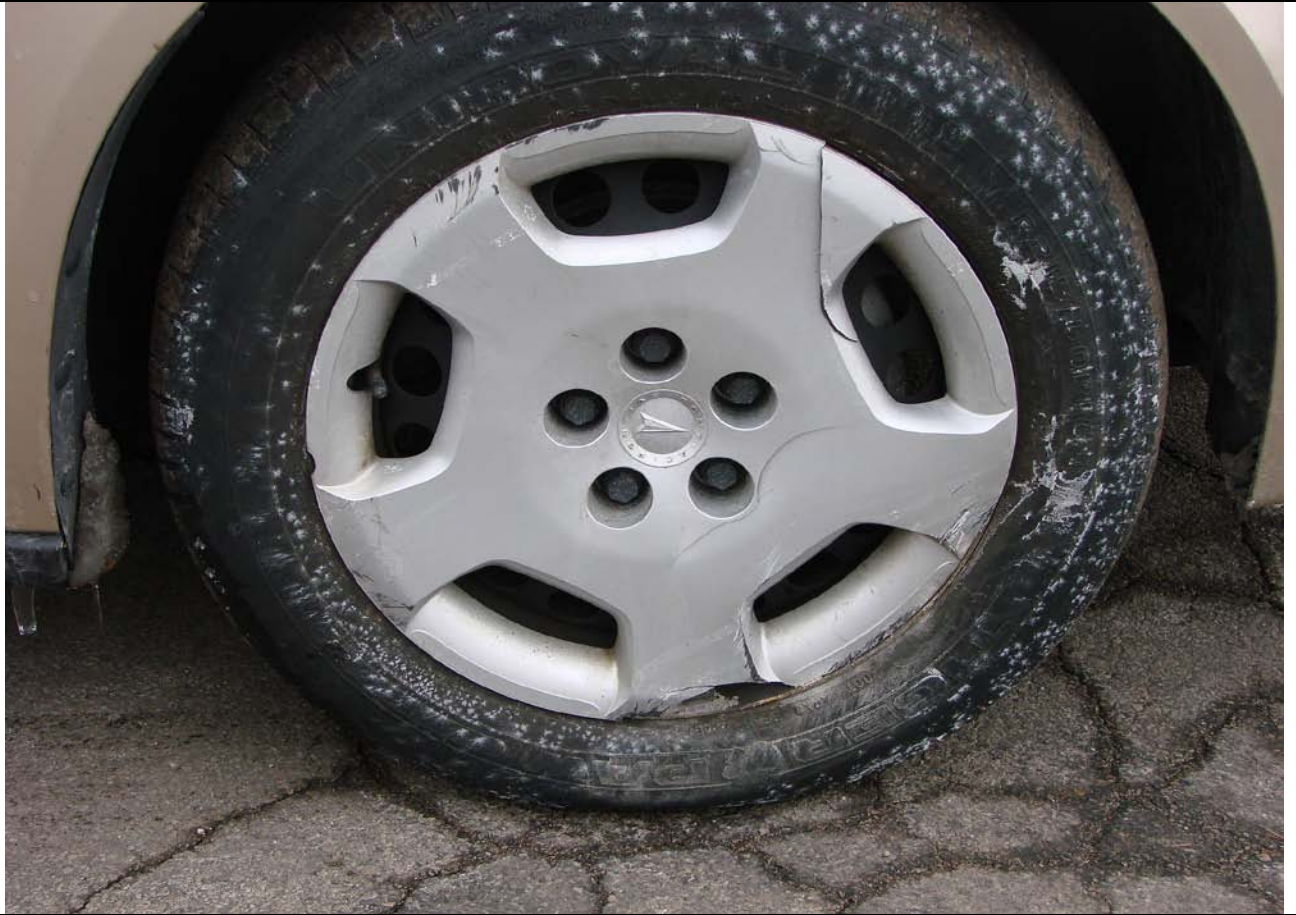
10 Damage to the RF wheel and wheel cover
