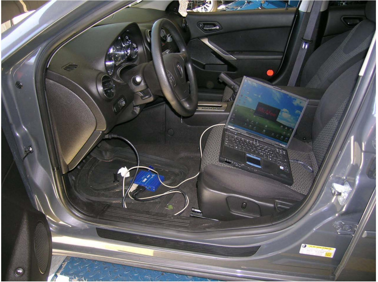
85. Tech 2 connected to the vehicle
