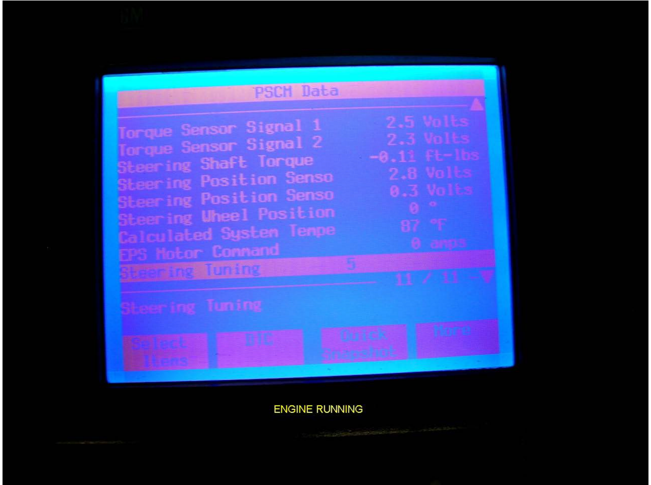
97. Tech 2 screen showing PSCM data with the steering wheel turned to the right
