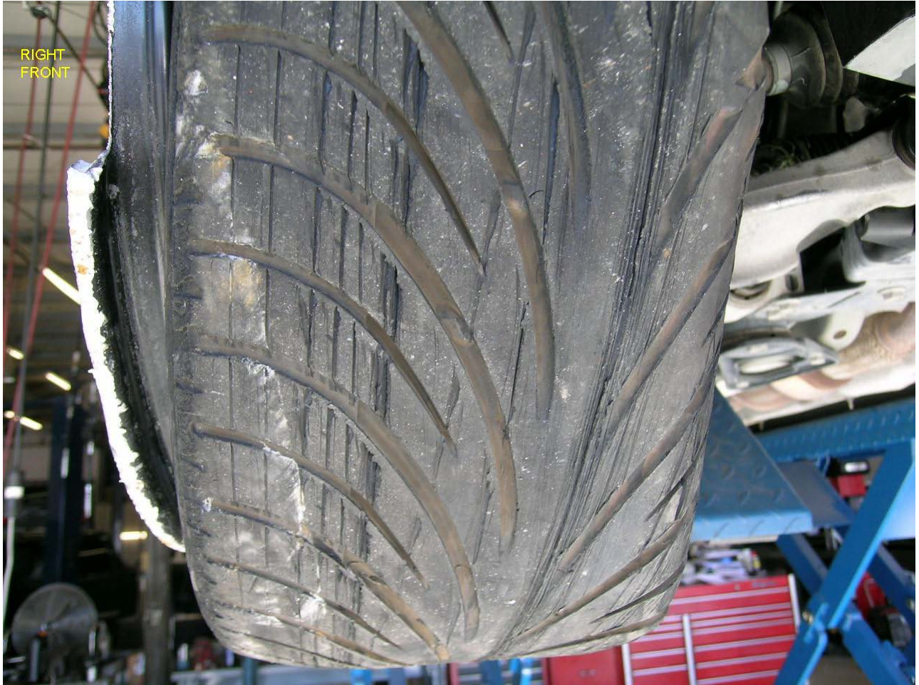
40. Overview of the outside of the right front tire and wheel showing damage and impact marks
