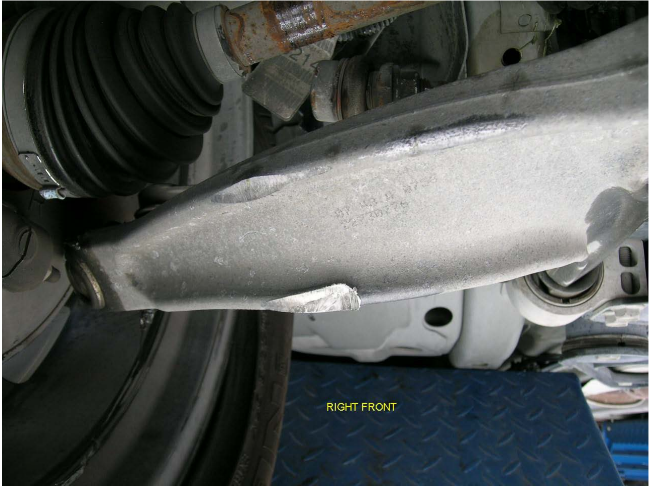
35. Closer view of the right front lower ball joint ball stud
