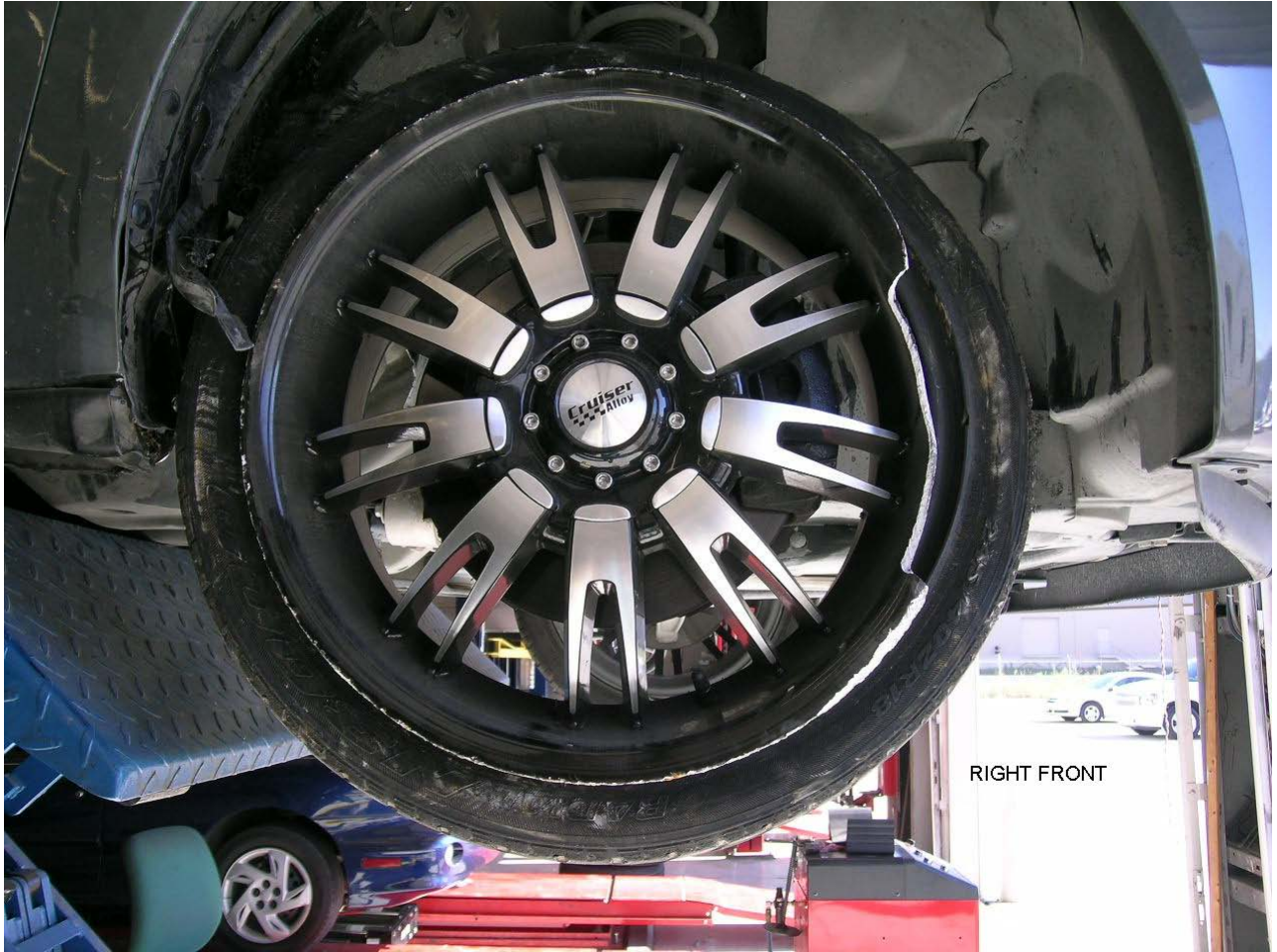
41. Front view of the damage to the outside of the right front wheel
