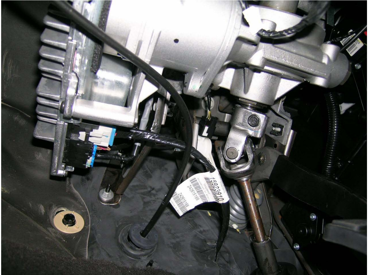
83. Closer view of the power steering motor harness connectors
