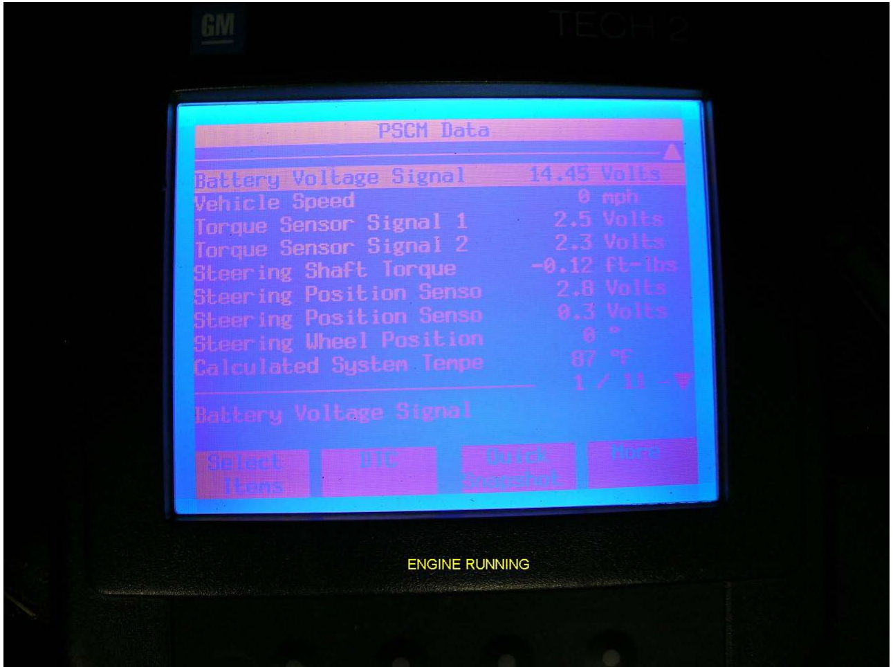
96. Tech 2 screen 2 of 2 showing PSCM data with the engine running
