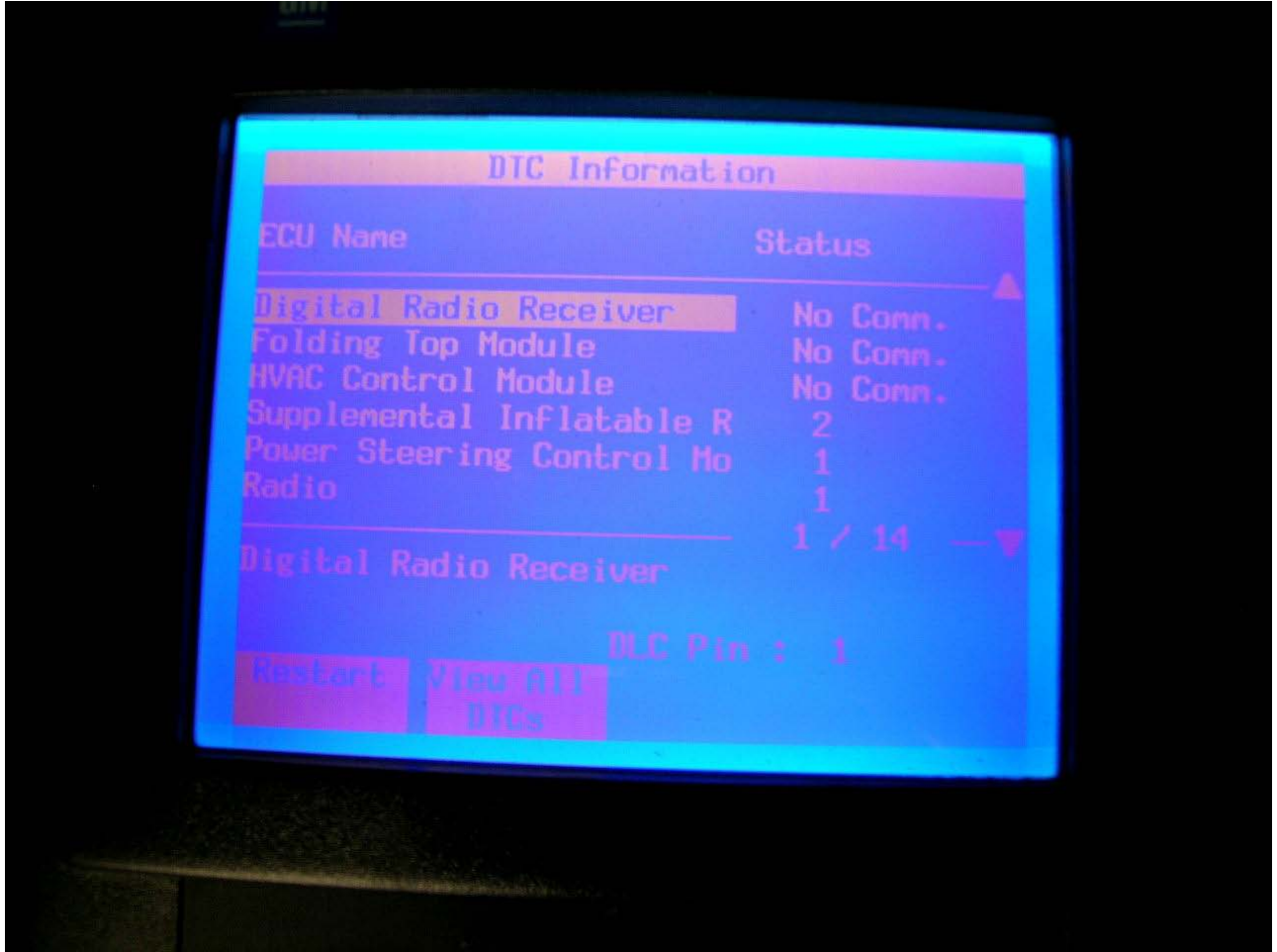
87. Tech 2 screen 2 of 3 showing DTC summary
