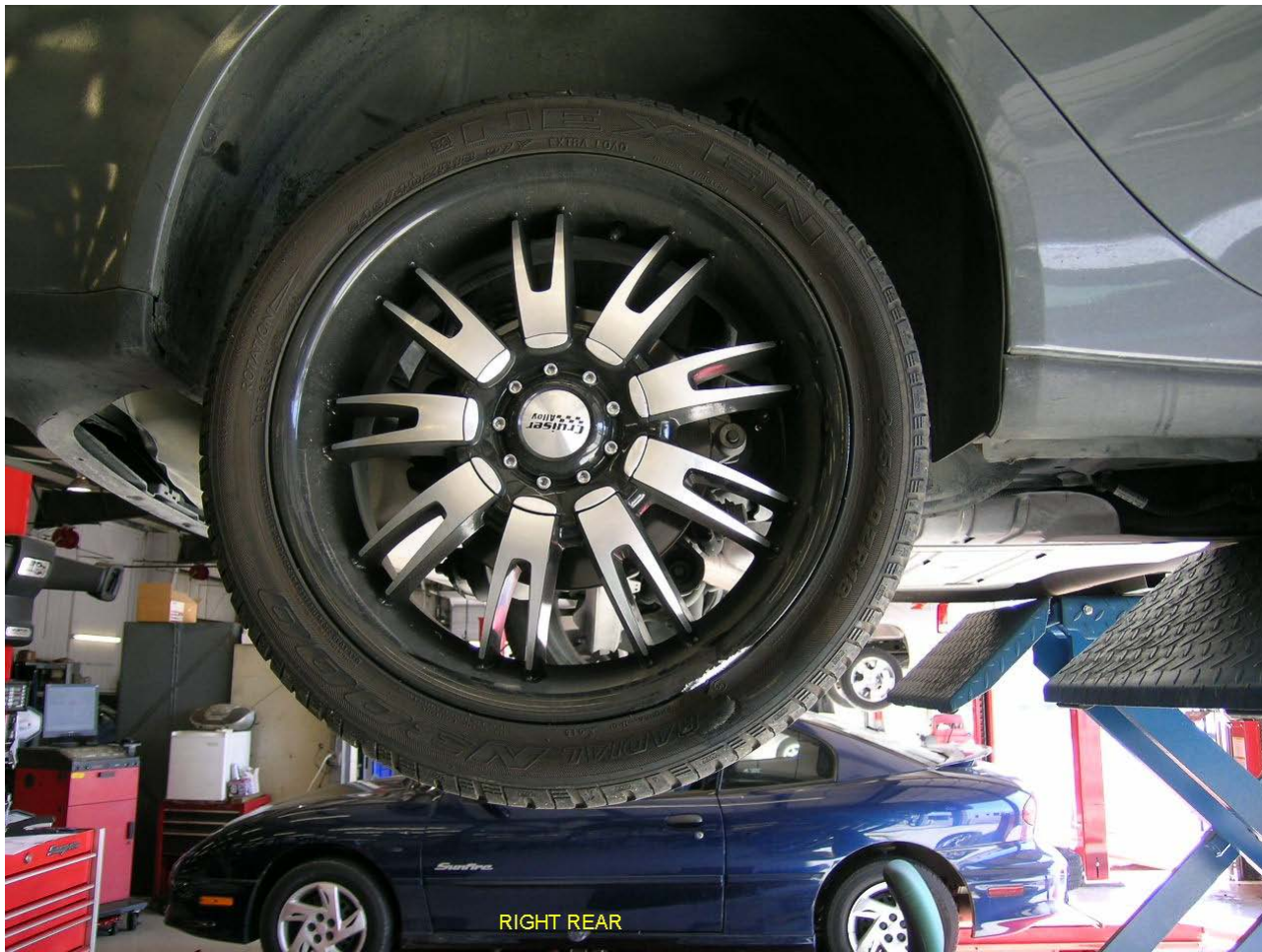
50. Closer view of the damage to the right rear wheel outer edge and the tire, showing impact mark
