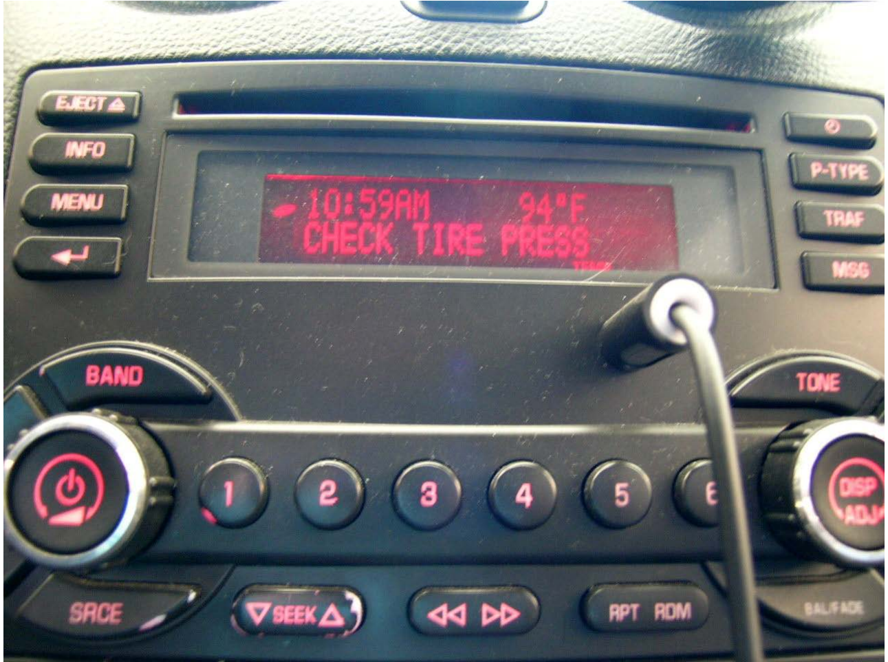
7. Front tire pressures showing in message center
