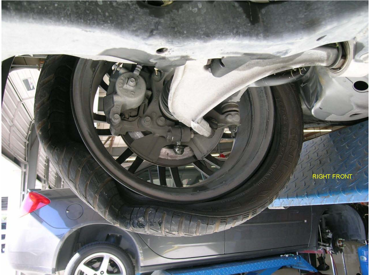
34. Impact marks on the right front lower control arm and scrapes on the drive axle
