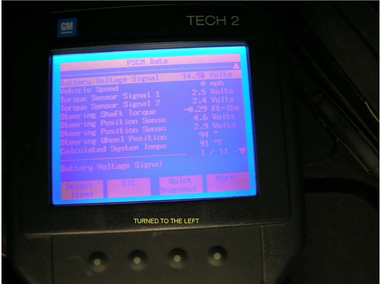
99. Tech 2 screen showing PSCM module information
