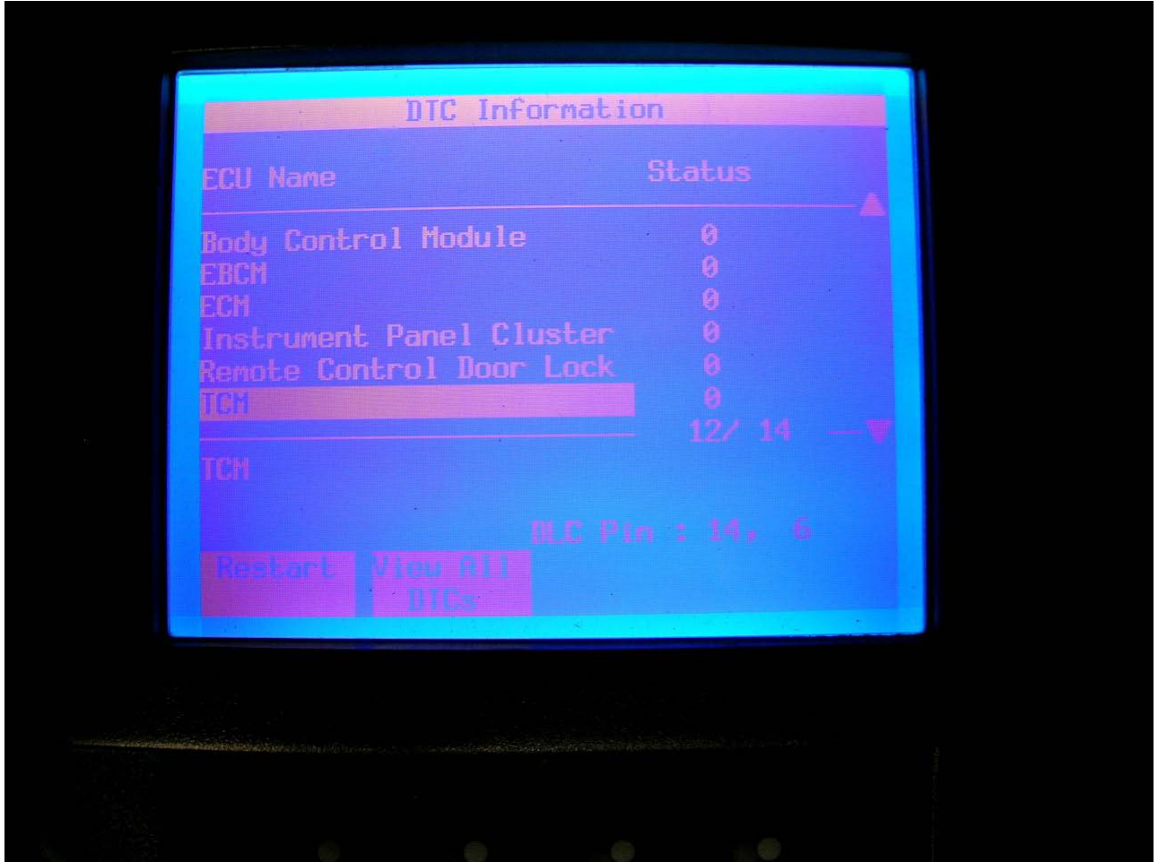
88. Tech 2 screen 3 of 3 showing DTC summary
