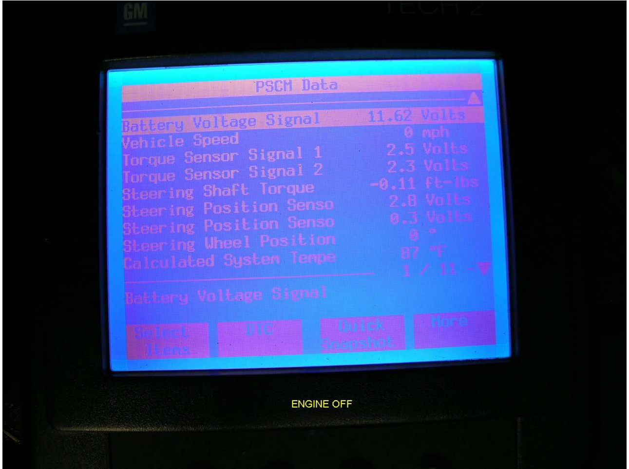
94. Tech 2 screen 2 of 2 showing PSCM data with the engine off
