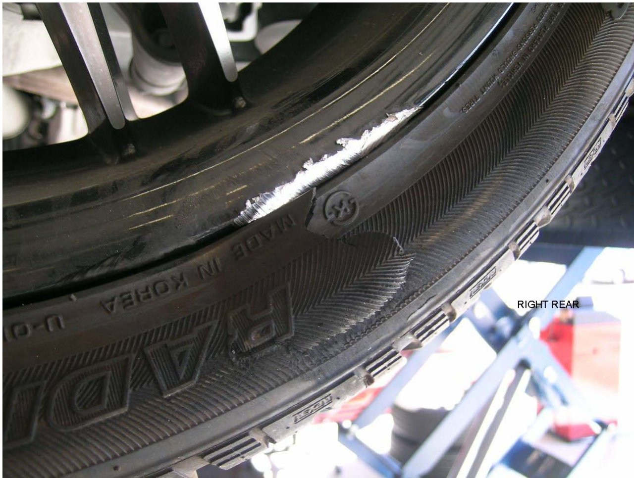
51. Closer view of the damage to the right rear wheel outer edge and the tire, showing impact mark
