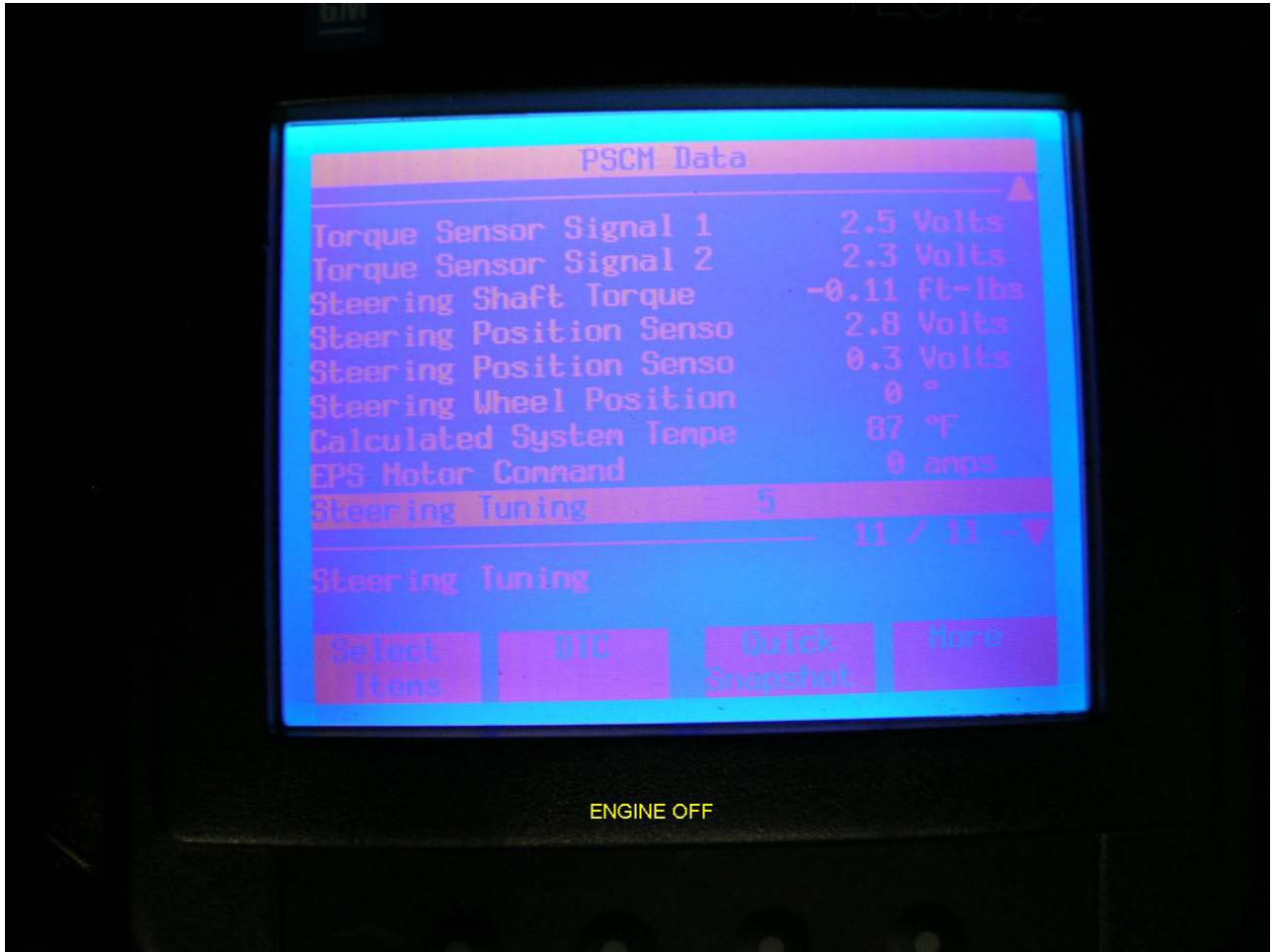
95. Tech 2 screen 1 of 2 showing PSCM data with the engine running
