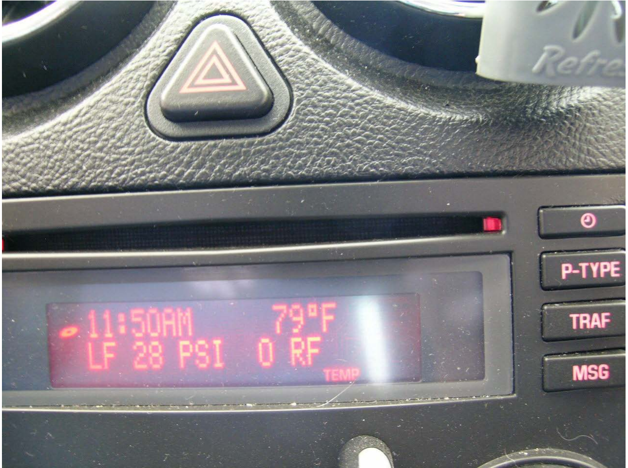
8. Rear tire pressures showing in message center
