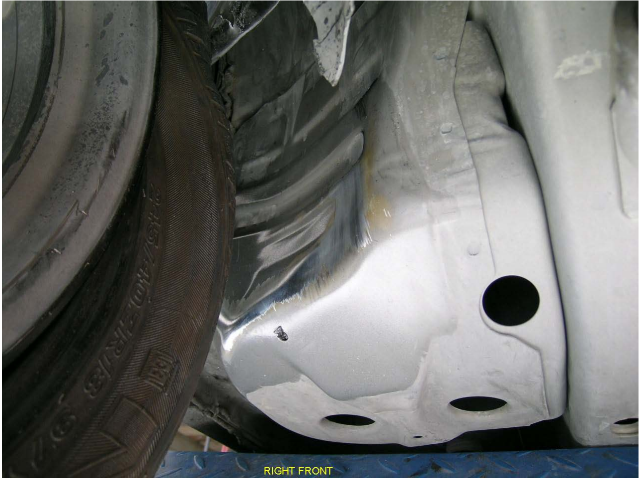
46. Closer view of the body damage at the rear of the right front fender
