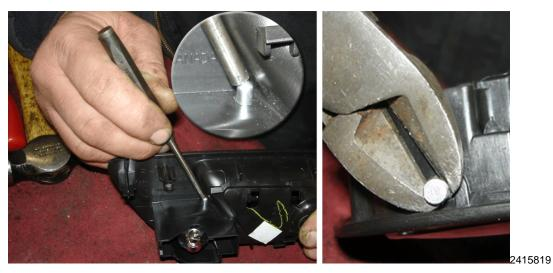
**Note:** Using a punch and hammer, strike the rounded end of the roll pin to loosen the roll pin. The head of the roll pin should protrude from the handle housing. Remove the roll pin with pliers as shown in the illustration.
