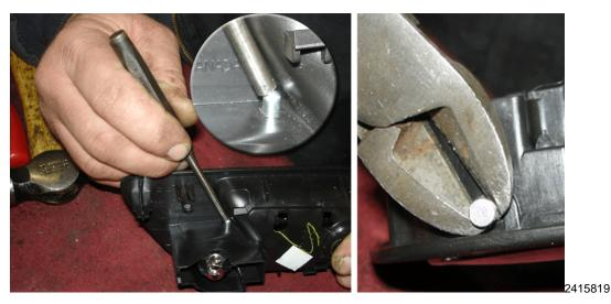
**Note:** Using the punch and hammer, strike the rounded end of the roll pin to loosen the roll pin. The head of the roll pin should protrude from the handle housing. Remove the roll pin with pliers as shown in the illustration.
