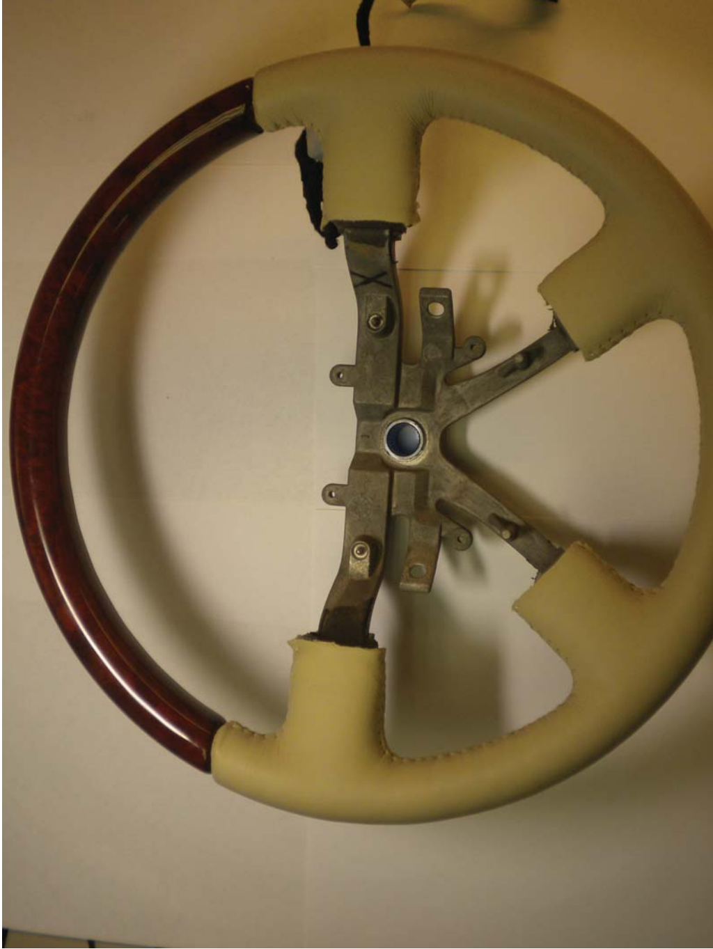
Front view of U231/U228 (Aviator/Navigator) Steering Wheel (back cover removed for visibility)
