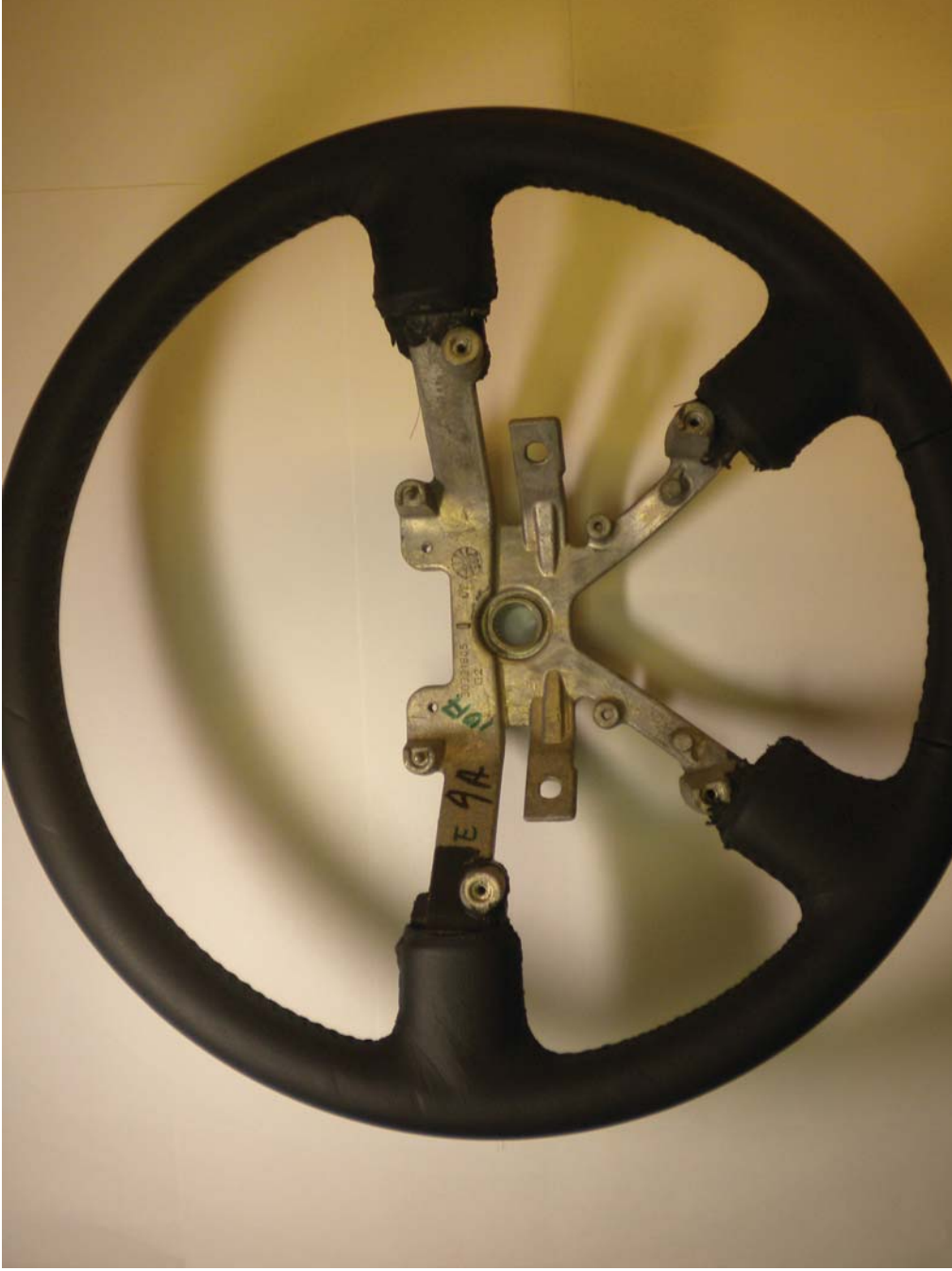
Front view of U152 (Explorer) Steering Wheel (back cover & switches removed for visibility)
