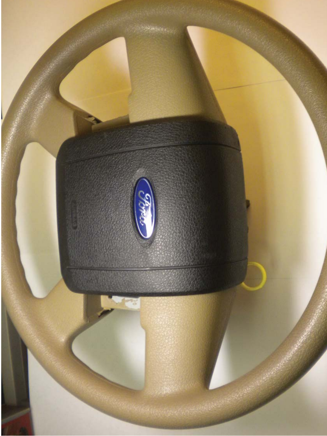
Angled view of P221 (F150) DAB installed into Str Whl
