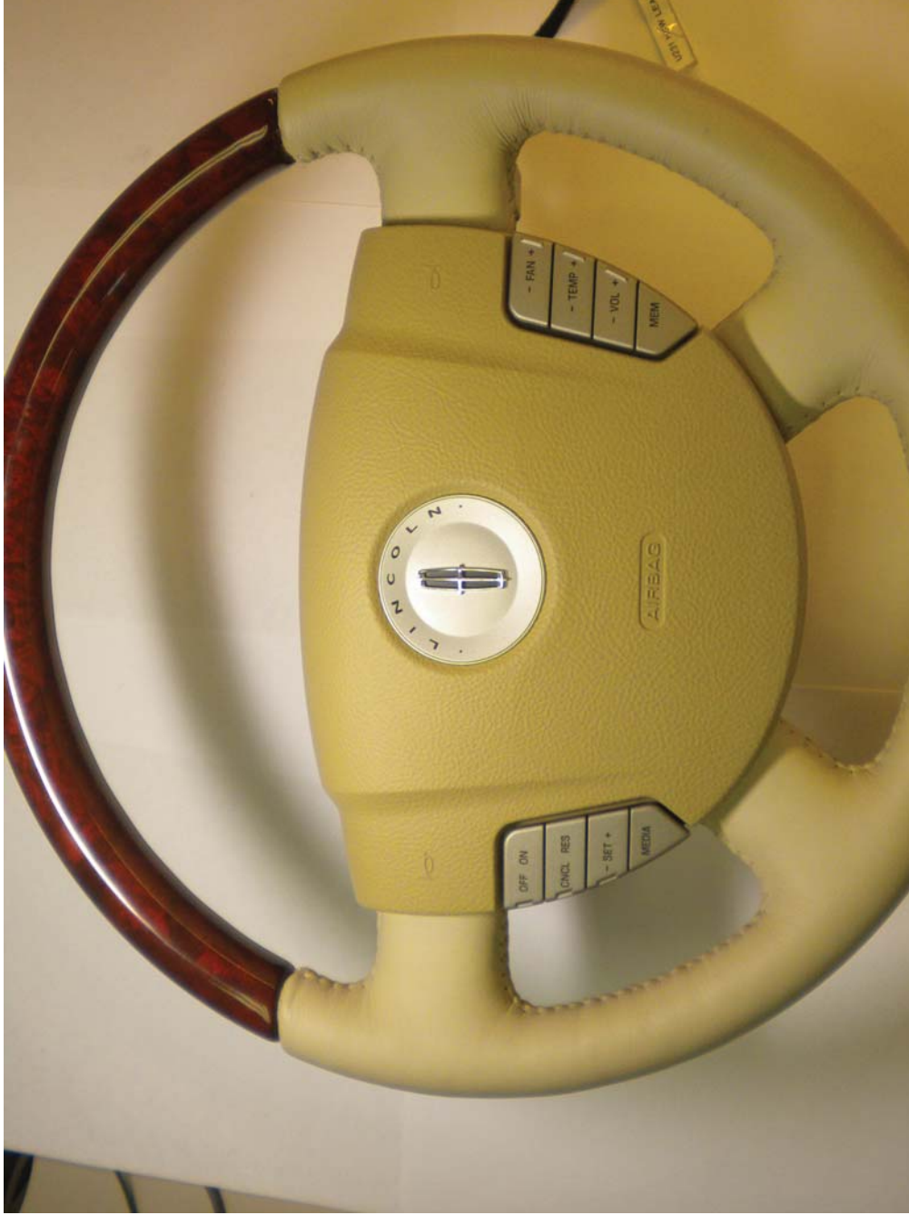
Front view of U231/U228 (Aviator/Navigator) DAB installed into Str Whl
