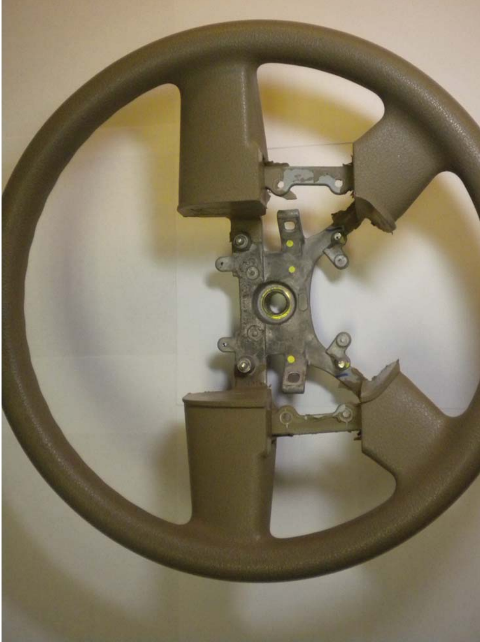
Front view of P221 (F150) Steering Wheel (back cover & switches removed for visibility)
