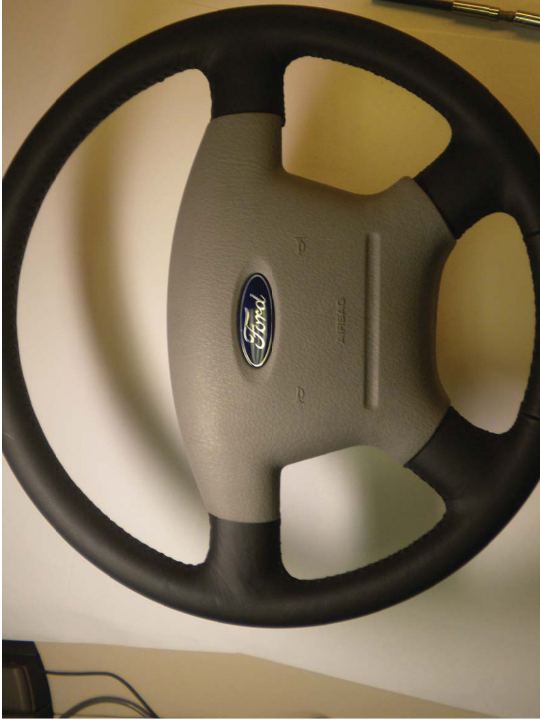
Front view of U152 (Explorer) DAB installed into Str Whl
