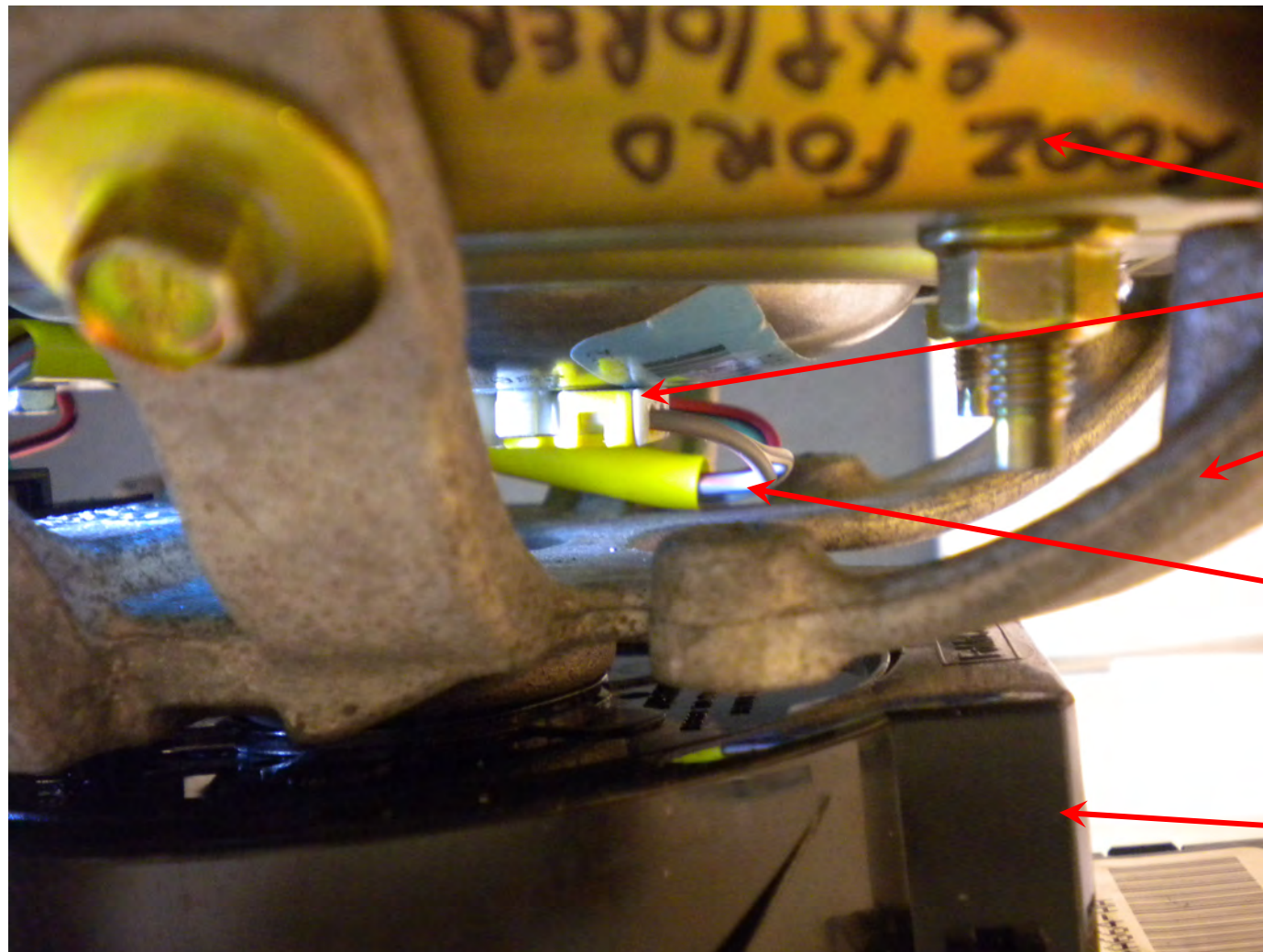
Left side view of clock spring, Str Whl, DAB
