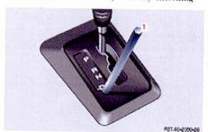
In the case of power failure the transmission selector lever can be manually unlocked, e.g. to tow the vehicle.
