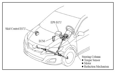
Figure 2. Toyota Corolla EPS components.
