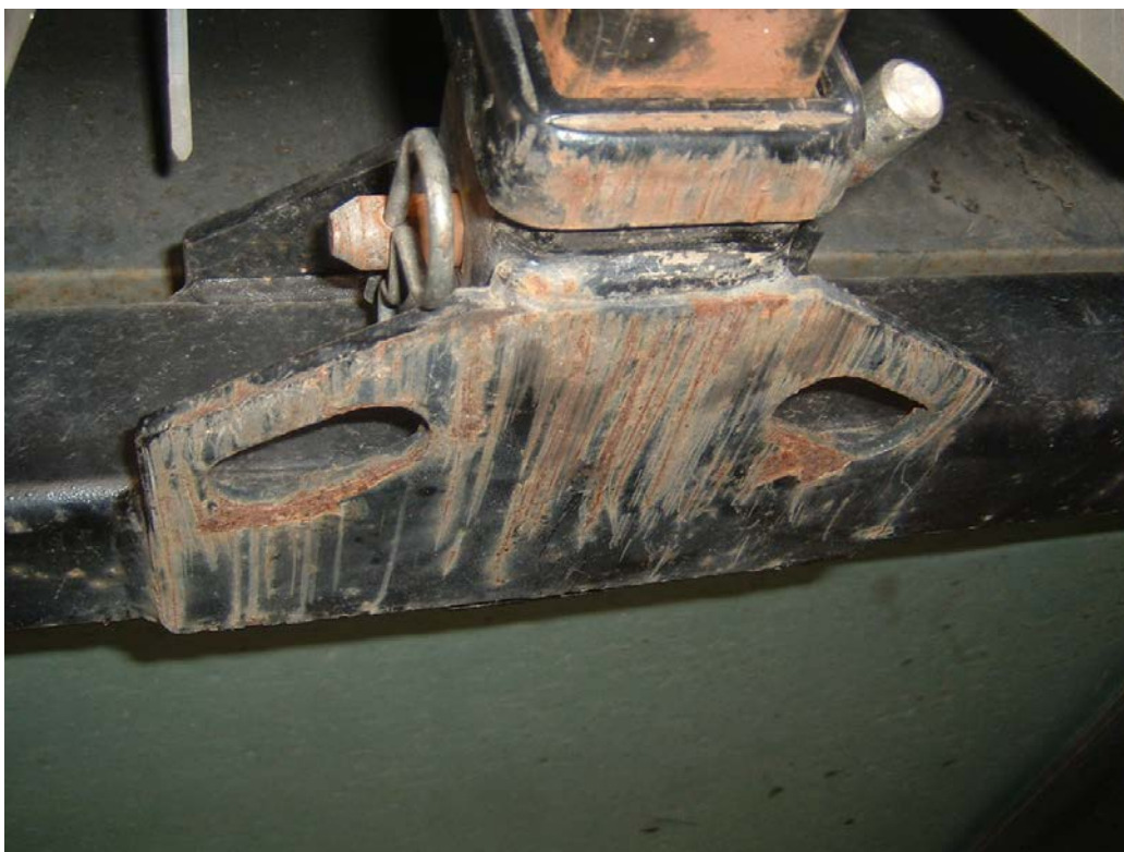
Photograph 5 - Bottom face of the hitch receiver plate that had been installed in the 2006 Winnebago Itasca vehicle described in VOQ 10368002.
