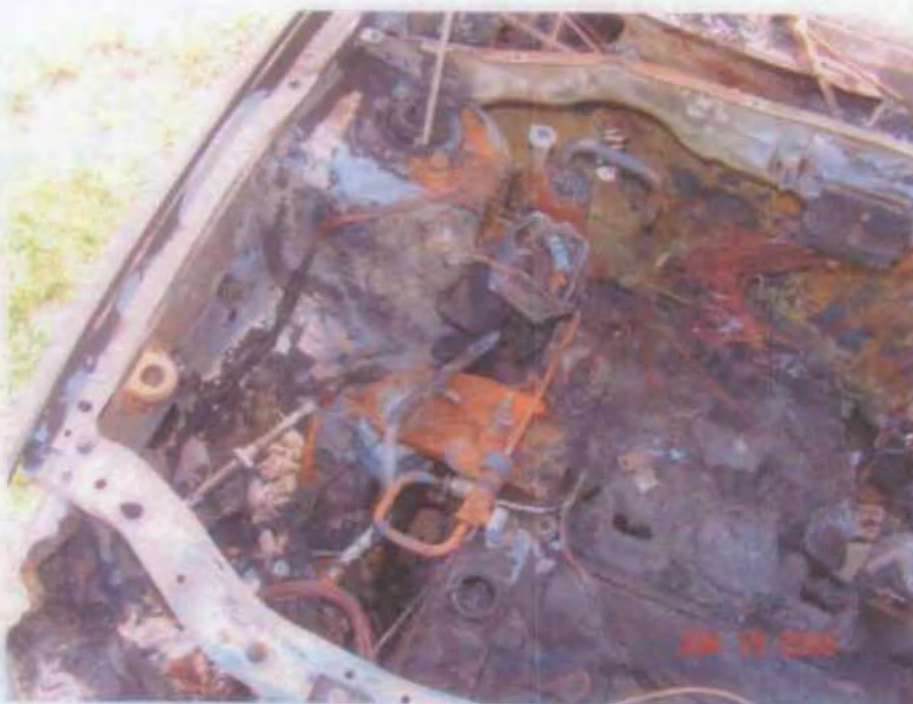
Photo 12 Photograph showing the large amount of damage to the passenger's side of the engine compartment
