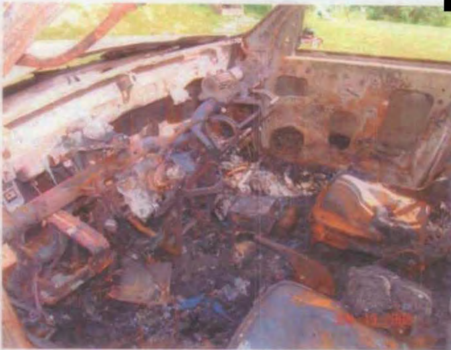
Photo 7 Photograph taken showing the very heavy damage to the interior from the driver's side
