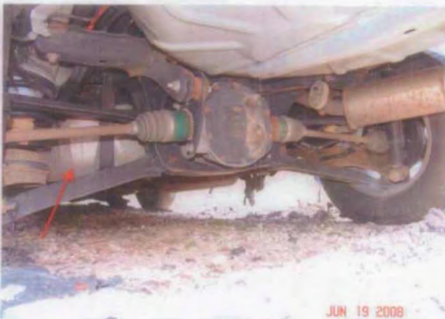
Photo 16 Photograph taken showing no signs of any fire damage to the under carriage or fuel tank
