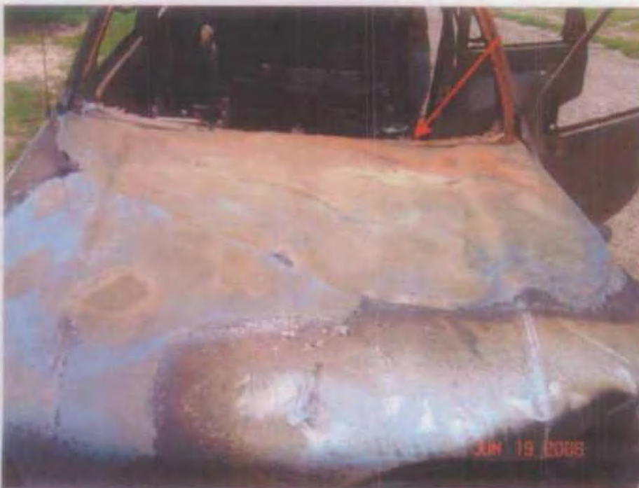
Photo 6 Photograph taken showing the fire pattern on the hood with the heaviest damage near the rear of the hood above the area where the heaviest damage was within the engine compartment
