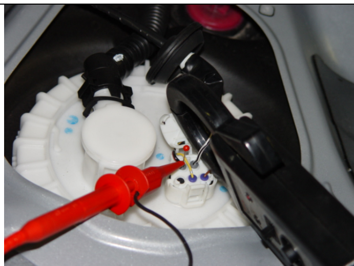
Voltage and electrical current were measured at Fuel pump module connector Pin#4 and Pin#5.
