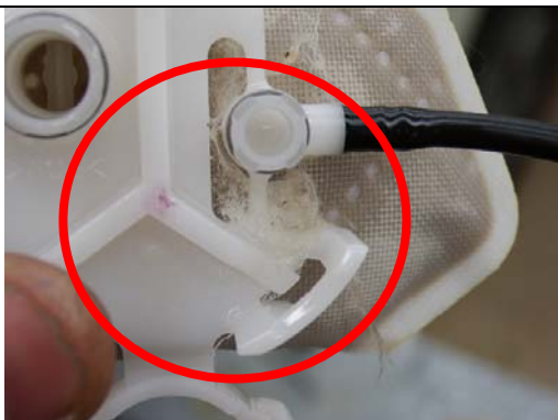
Fuel Pump pick up contaminated
