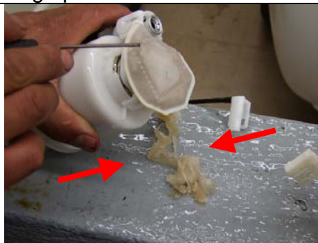
FOREIGN MATERIAL STUCK IN FUEL PICK UP
