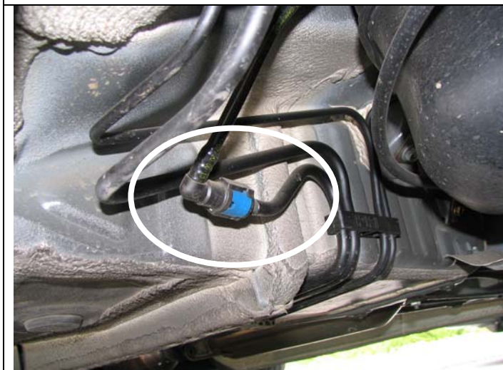
Fuel line connection located ahead of the left-rear wheel.
