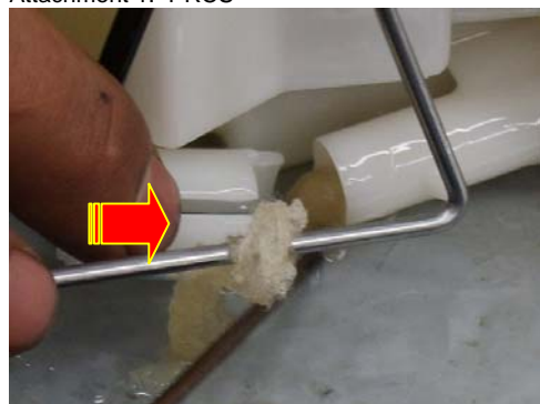
Fuel Pump pick up contaminated
