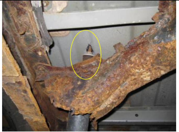
This photo is of the mount from a different angle. Here the shock can be seen penetrating the bed.
