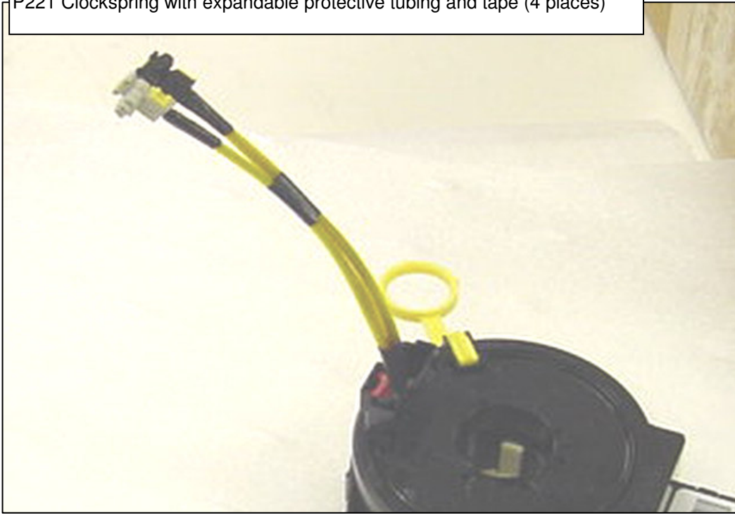
P221 Clockspring with expandable protective tubing and tape (4 places)
