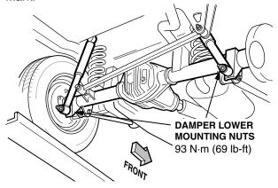
6. Torque the lateral rod-to-axle mounting nut to 93 N⋅m (69 lb-ft). Mark the nut and bolt with the Brite-Mark.
