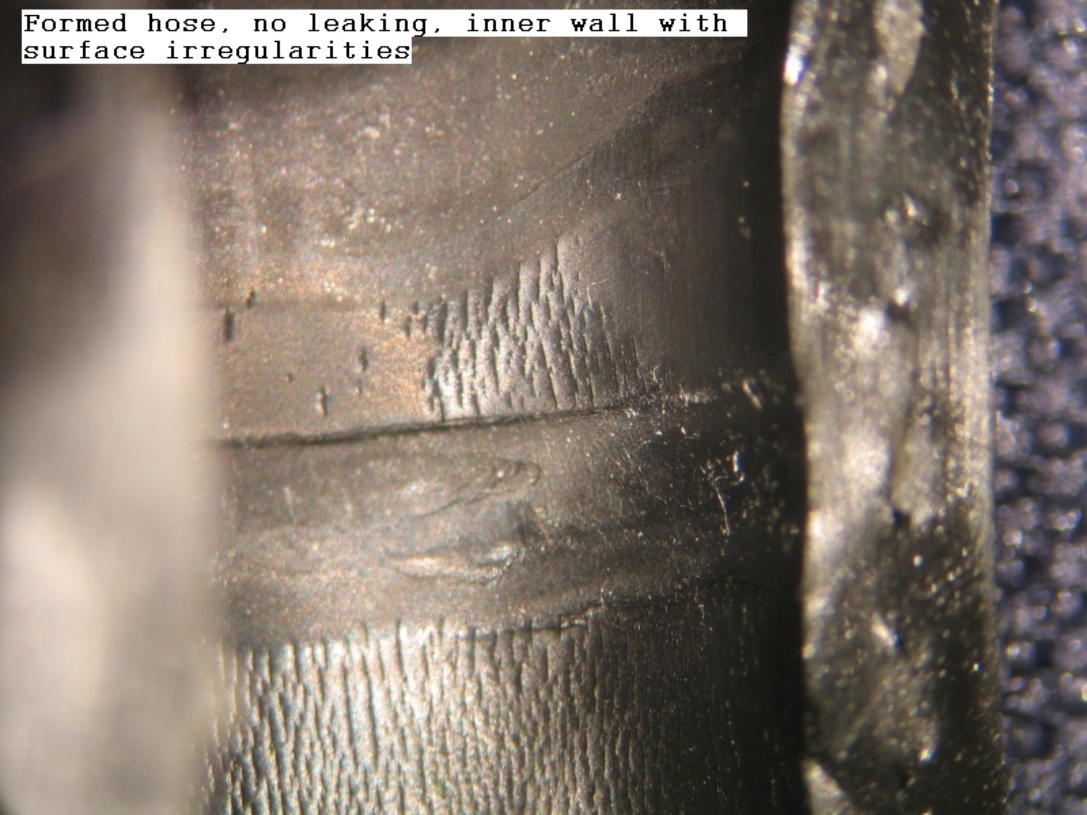
Formed hose, no leaking, inner wall with surface irregularities, small cracks in "clip" areas
