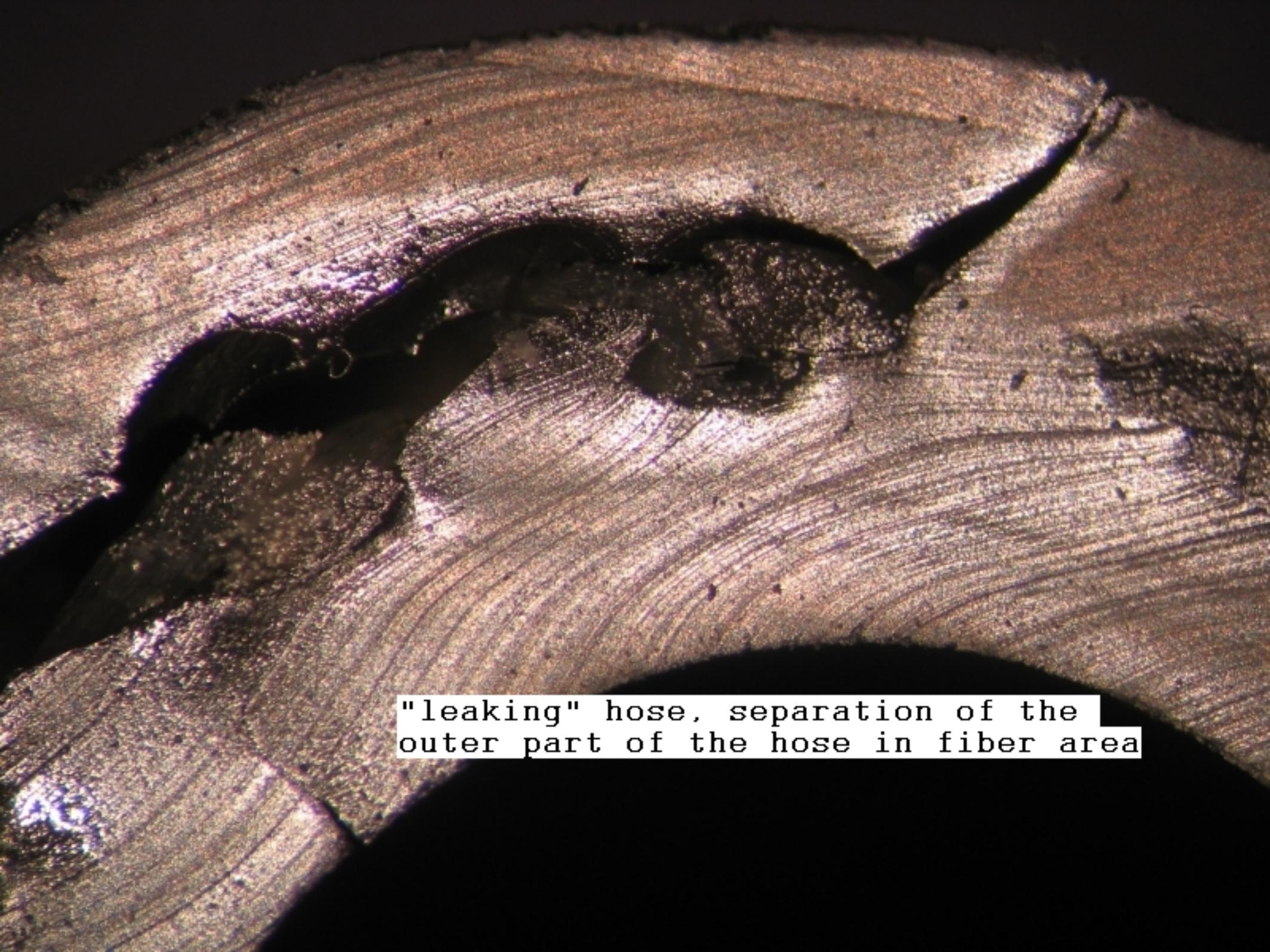
"leaking" hose, separation of the outer part of the hose in fiber area
