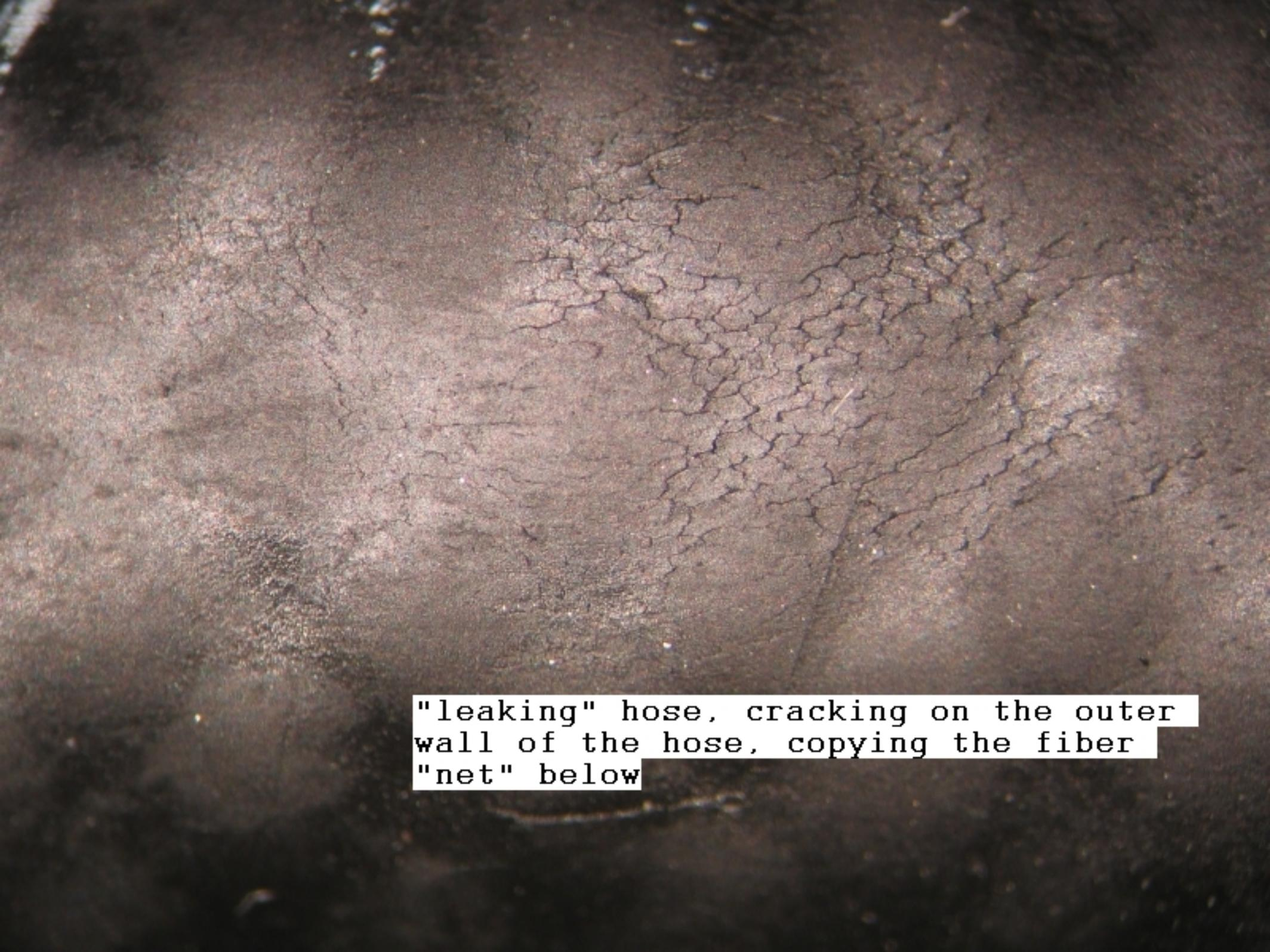
"leaking" hose, cracking on the outer
