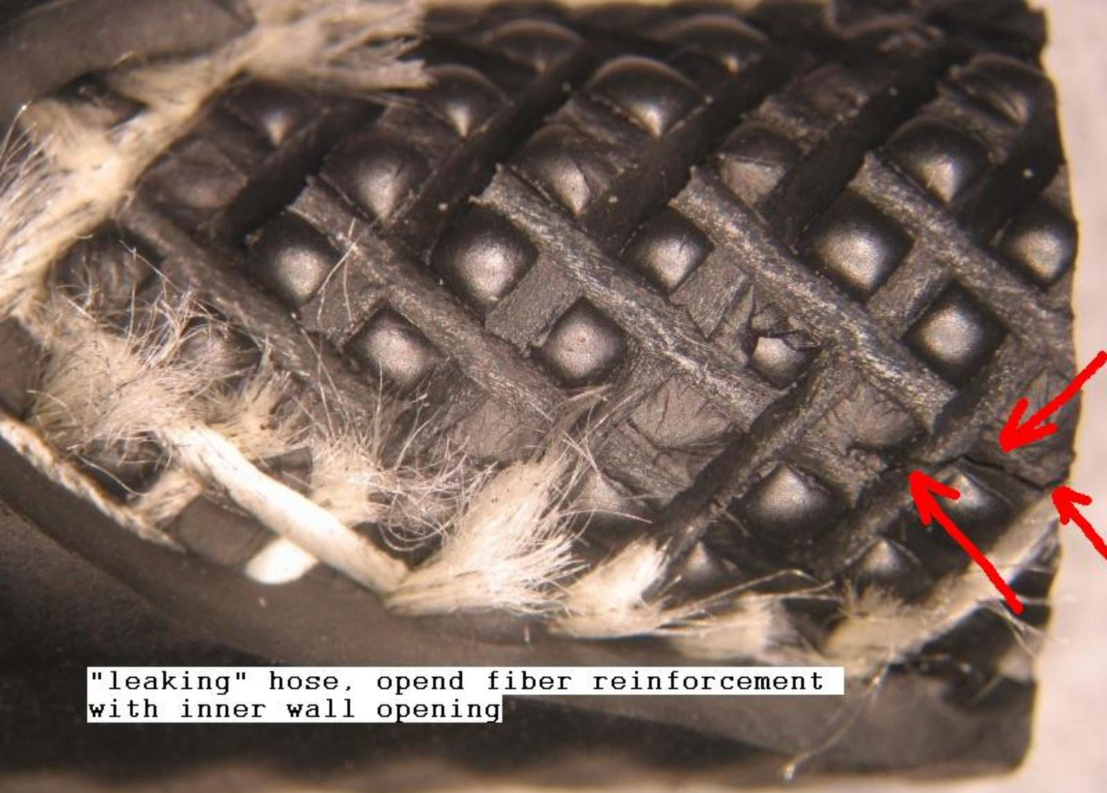
"leaking" hose, opened fiber reinforcement with inner wall opening
