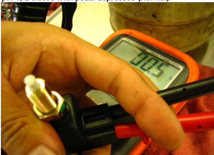
(A) pin 1, 2 closed with pedal depressed (normal)
