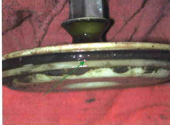
The piston o-ring groove area shows oil contaminates residue.
