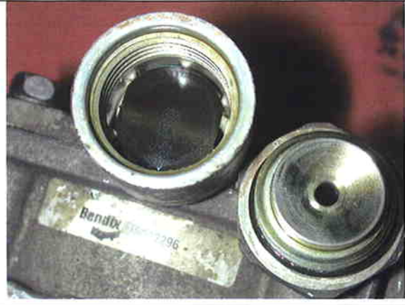
Excessive oil contamination inside the service quick release cavity
