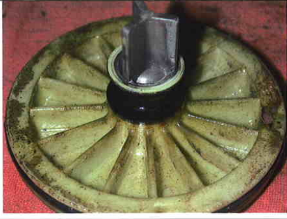
Control piston's delivery side shows excessive oil and grit contaminates.
