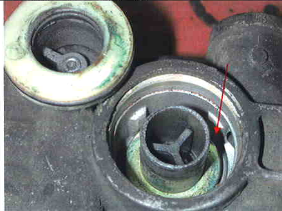
Exhaust inlet cavity shows less contaminates. Lacking grease.
