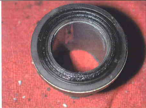
I/E valve seat shows excessive wear from oil mix grit contaminates.
