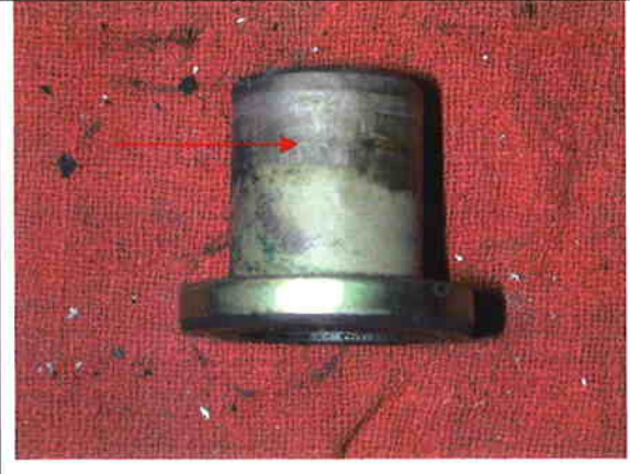
I/E valve OD surface lacks grease.
