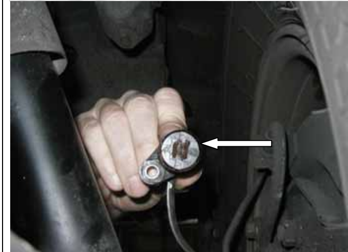
Debris found on the left rear speed sensor
