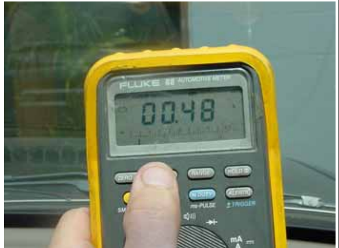
Minimum voltage recorded at the time brake malfunction indicator came on for tech. Within spec of good pedal stroke sensor and circuit.
