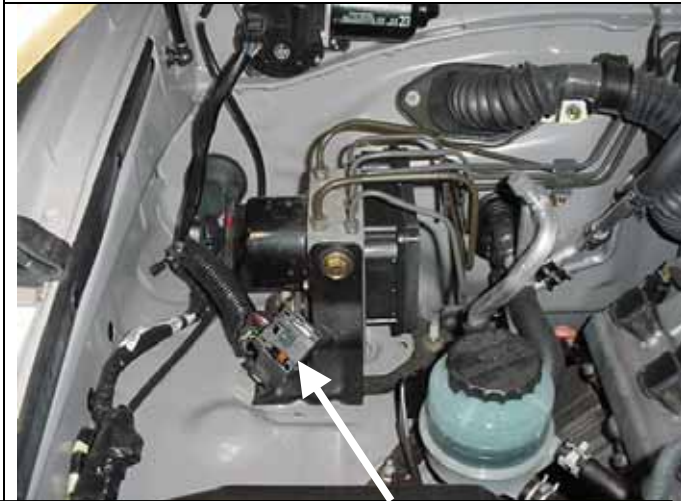
This is the skid control ECU with the connector unplugged.
