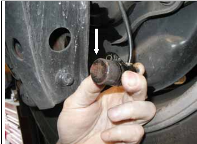
Debris on right rear wheel speed sensor
