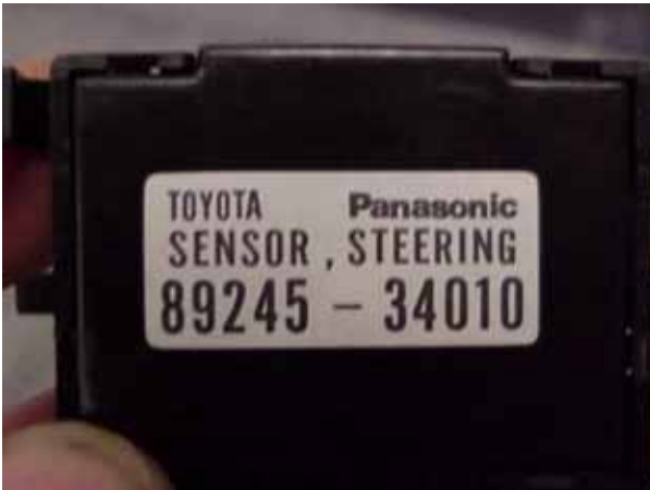
Photo of steering angle sensor and P/N.
