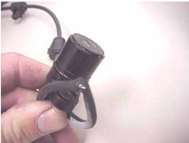
Wire harness damaged about 3 inches from sensor.
