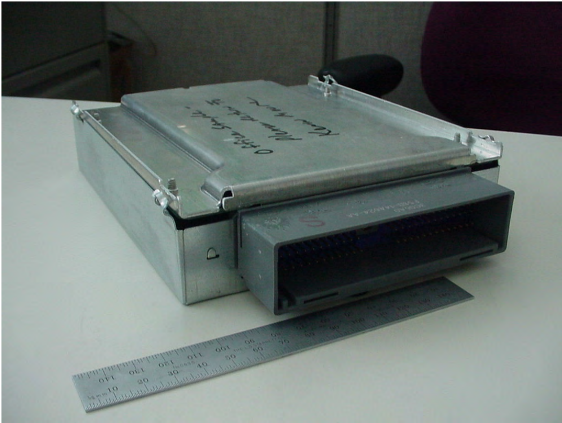
Figure 1. The V229 module with the cover slightly open to show the butt interface of the cover, the base, and the connector.
