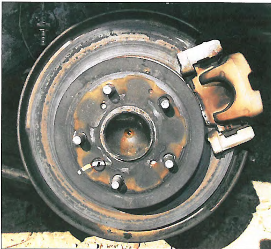
Figure 2 - Rear Left Caliper and Rotor Exhibiting Signs of Endured Braking
