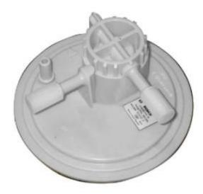
Inspect the entire flange surface for cracks and leakage if a fuel odor is present.
