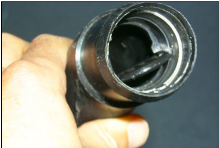
Figure 8: A flap valve installed closer to the tank in the filler tube.
