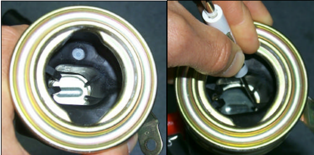
Figure 7: Flap valve found immediately behind the gas cap.
