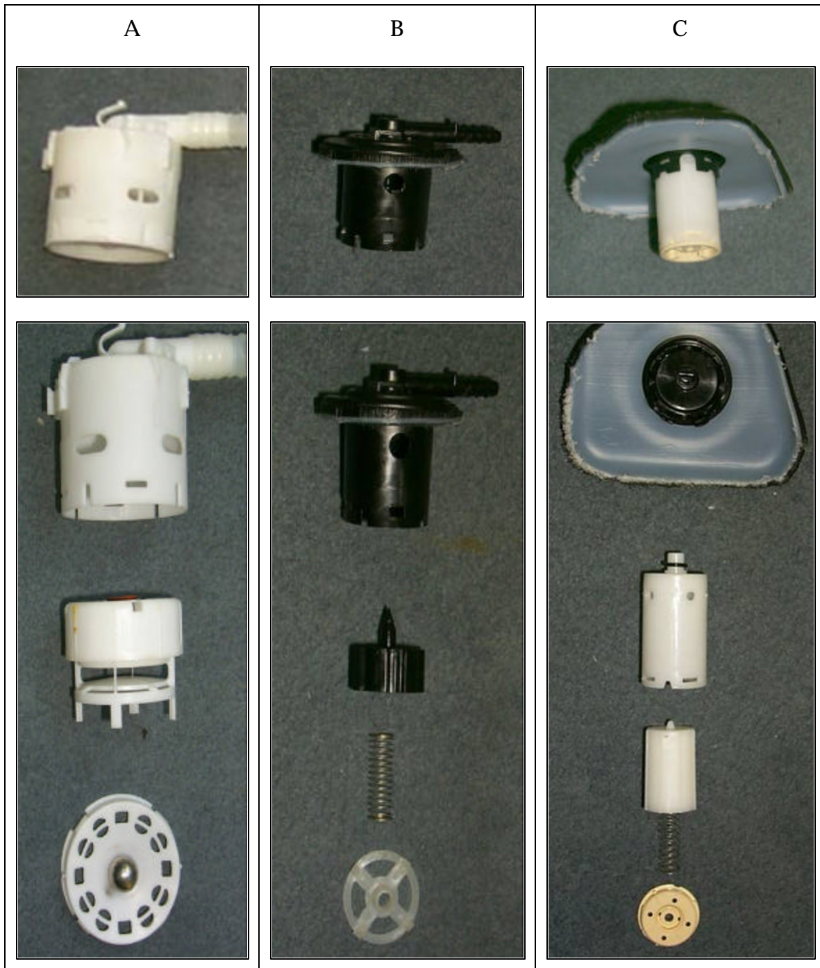
Figure 12: Examples of rollover valves from: a) Mercedes S430, b) Dodge Neon and c) Honda Odyssey.
