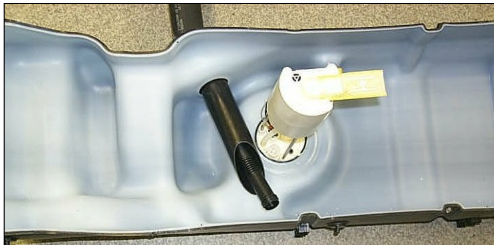
Figure 6: Cross-section of the upper half of a GMC Sierra gas tank.
