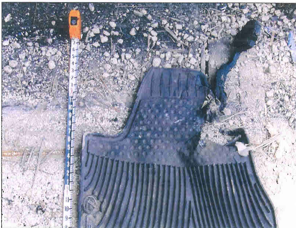
Figure 4 - All Weather Floor Mat Removed from Driver's Footwell, Bonded to Lower Edge of Accelerator Pedal Assembly
