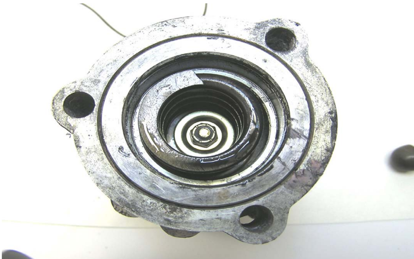
Steel Spring Adapter Assembly – Retainer Ring & Plunger Cap Removed
