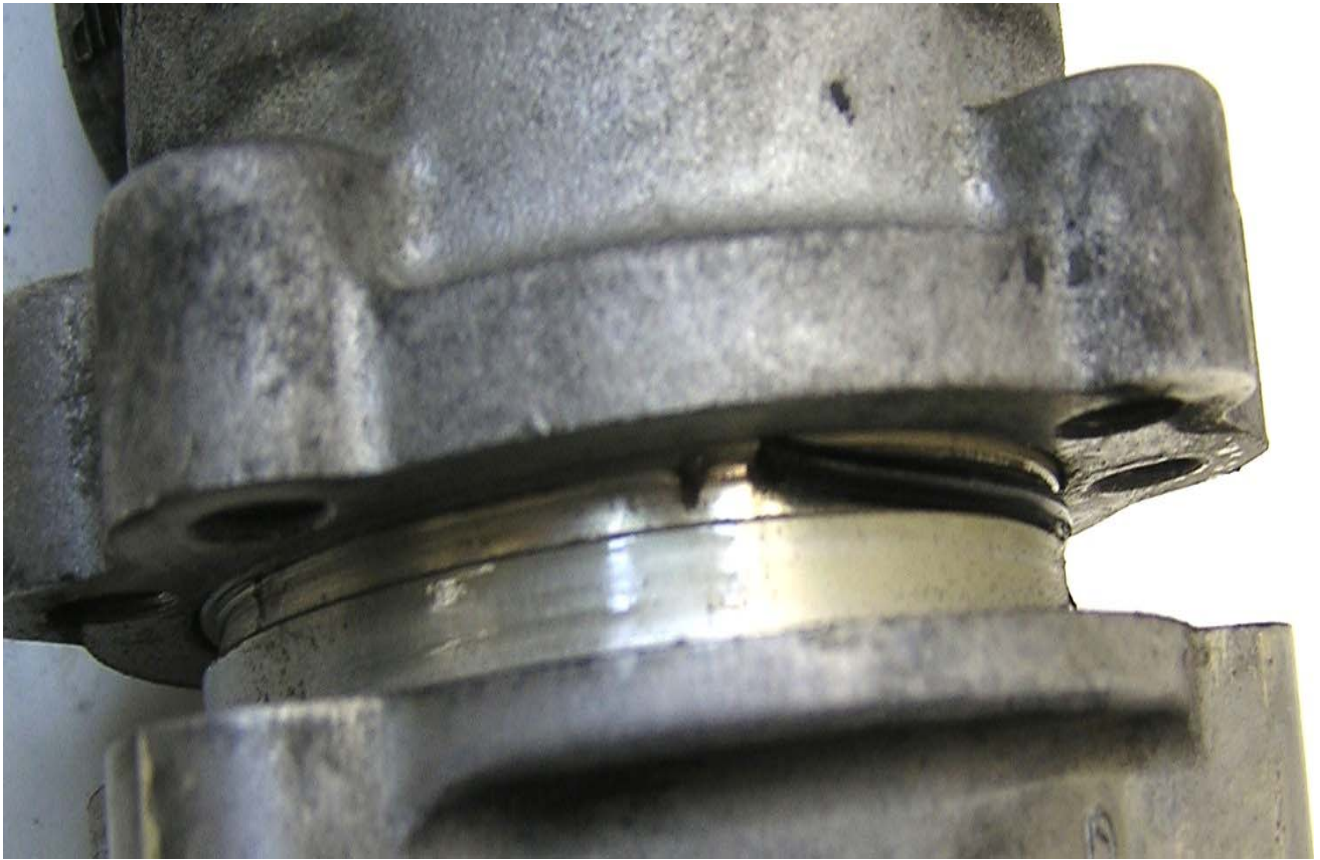
Steel Spring Adapter & Cut O-Ring
