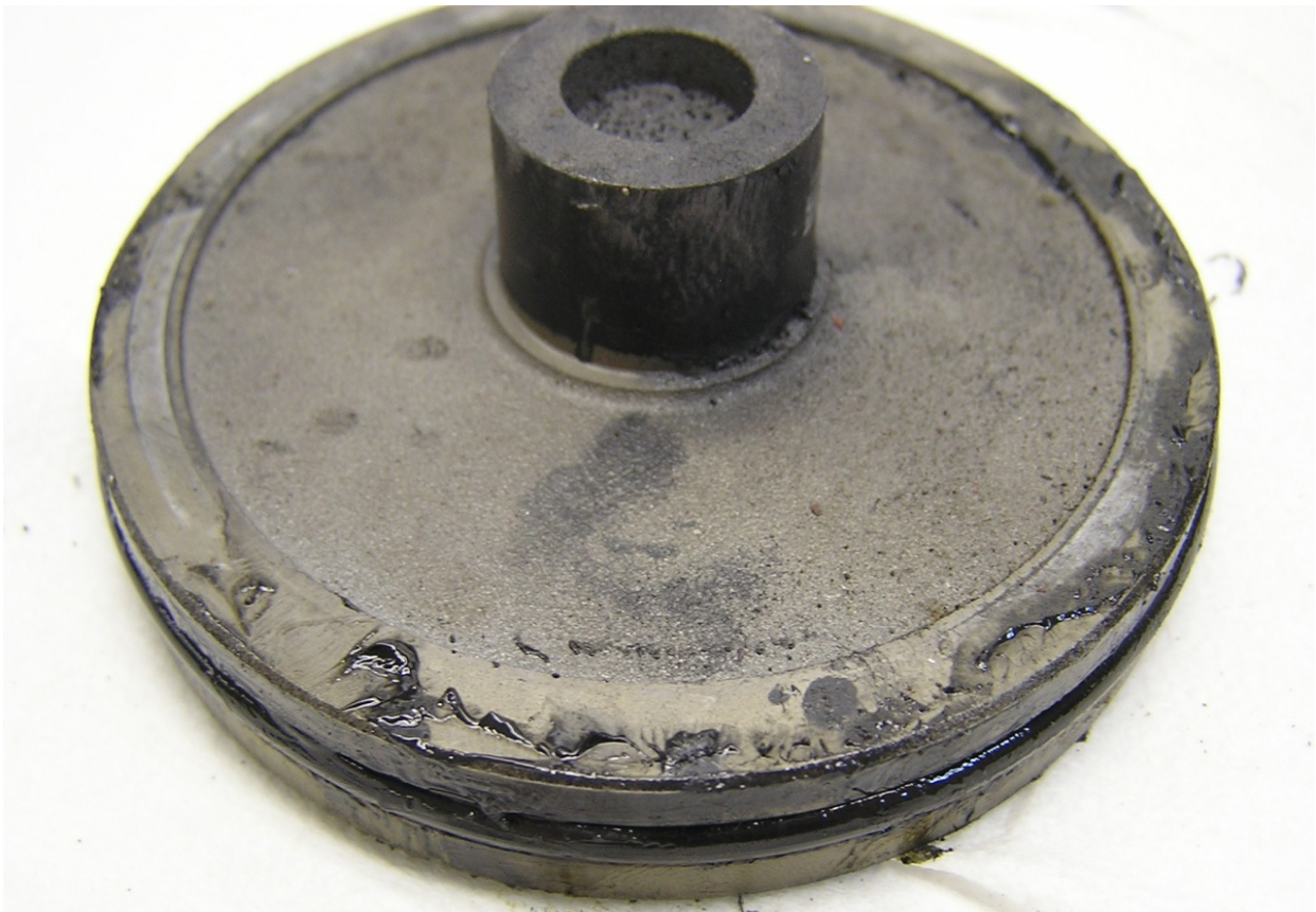
Top of Piston with Sticky Deposits
