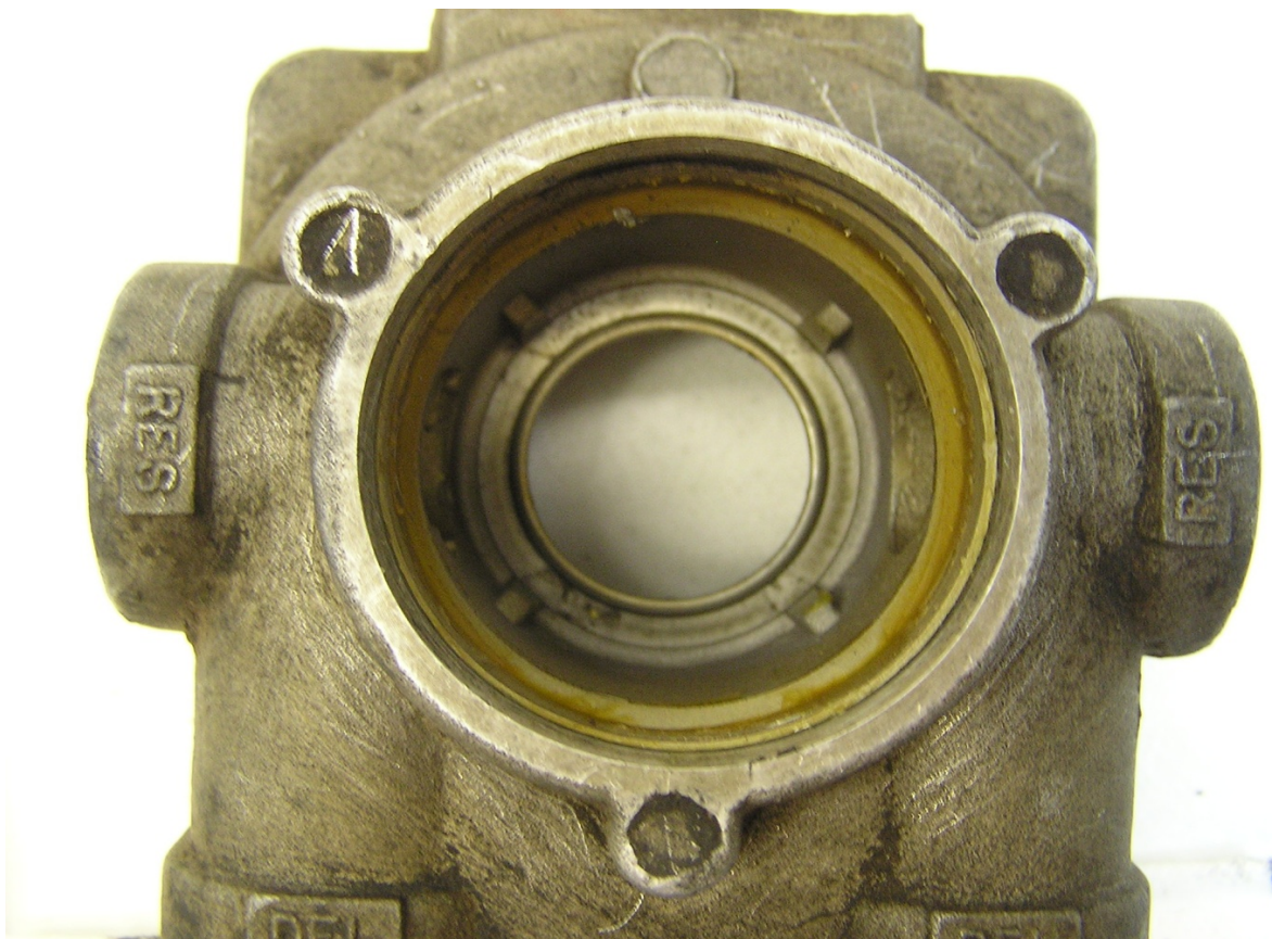
Supply Cavity and Supply Seat
