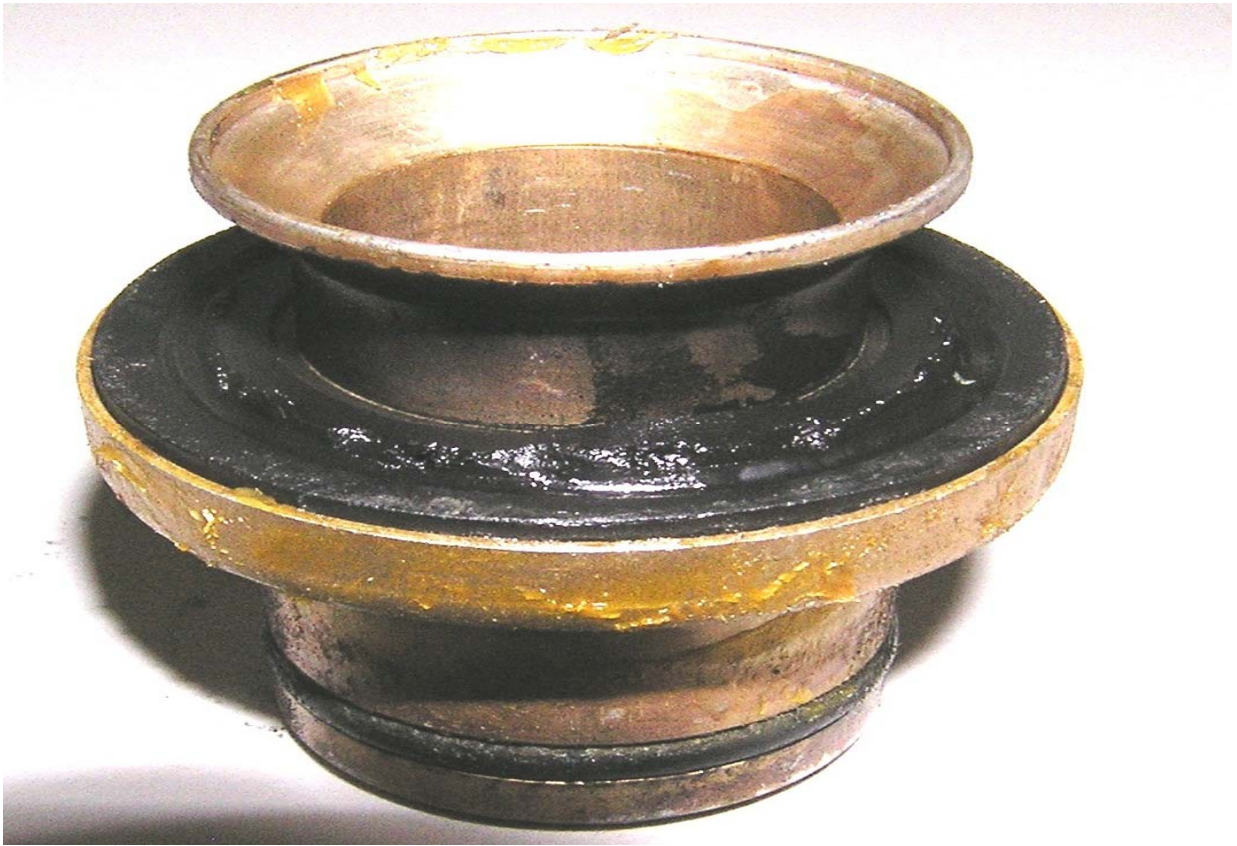
Modulation Tube with Inlet Seal and Exhaust Seat
