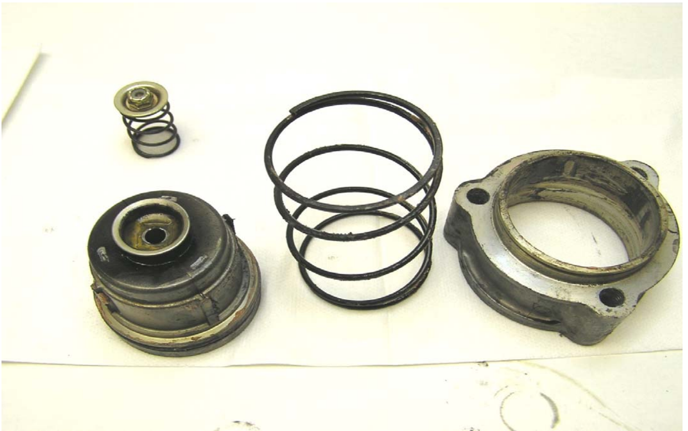
Primary Piston Underside with Springs & Adapter Body
