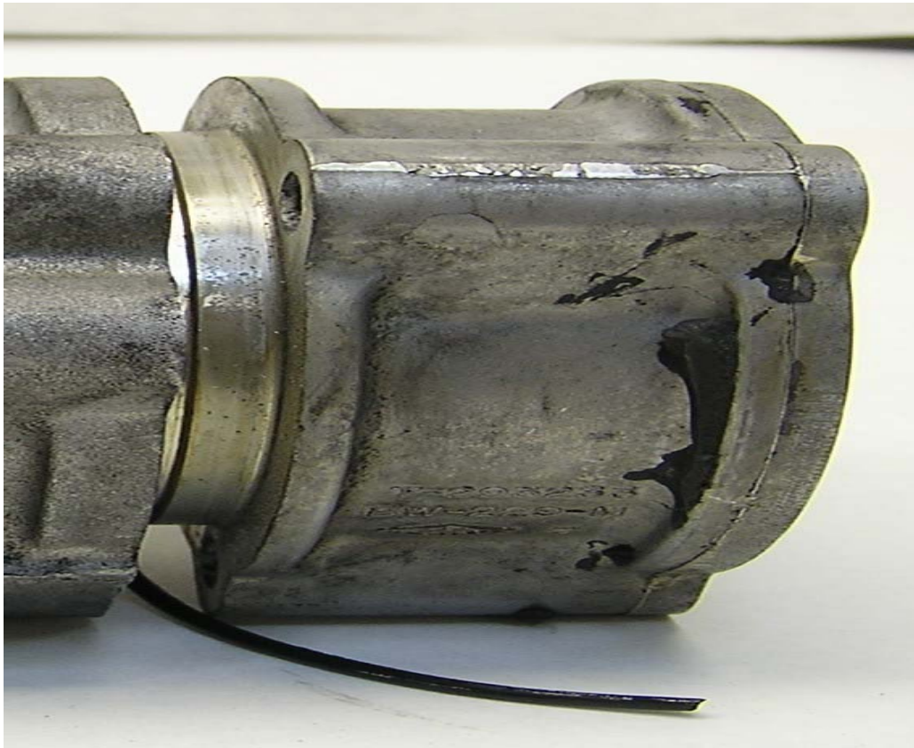
Steel Spring Adapter & Cut O-Ring
