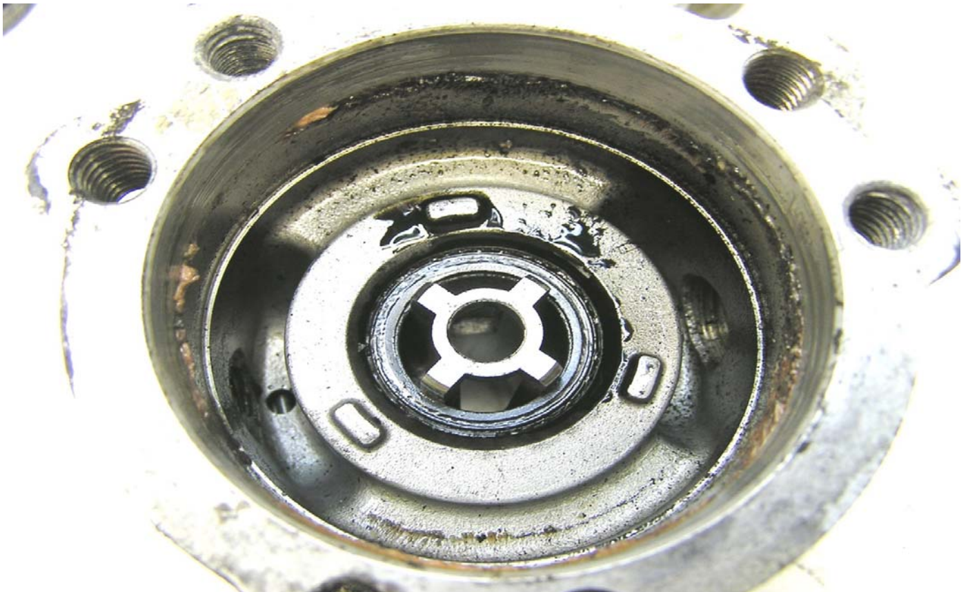
Primary Body Cavity with Primary Inlet/Exhaust Seal
